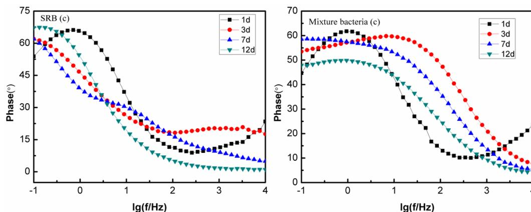
**Figure 2.** Nyquist and Bode diagrams of brass immersed in four media (a represents the Nyquist diagram, b represents the magnitude diagram, and c represents the phase-angle diagram)
