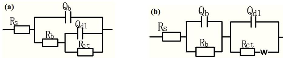
**Figure 3.** The equivalent circuit models used to fit the EIS experimental data for brass immersed in (a) sterile seawater system and single PAO-1 system, (b) single SRB system and composite system
