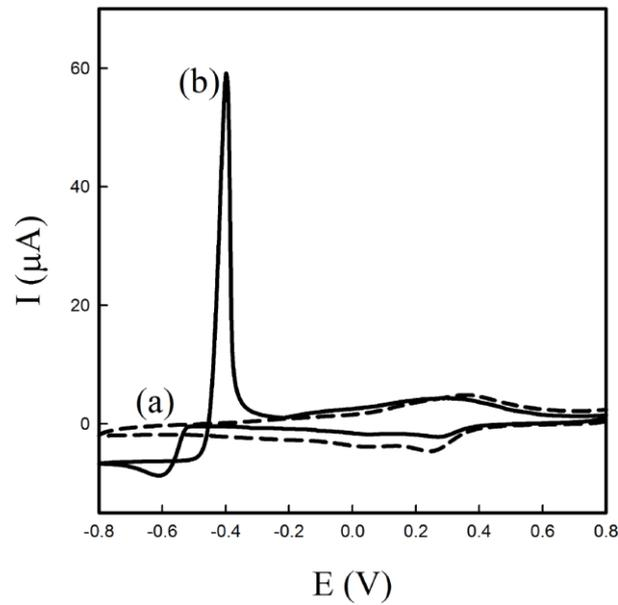
**Figure 3.** CV of the P(Ani-co-3ABSA) electrode (a) in 0.2 M potassium nitrate and (b) in  $1 \times 10^{-7}$  M  $\text{Pb}^{2+}$  plus 0.2 M potassium nitrate.
