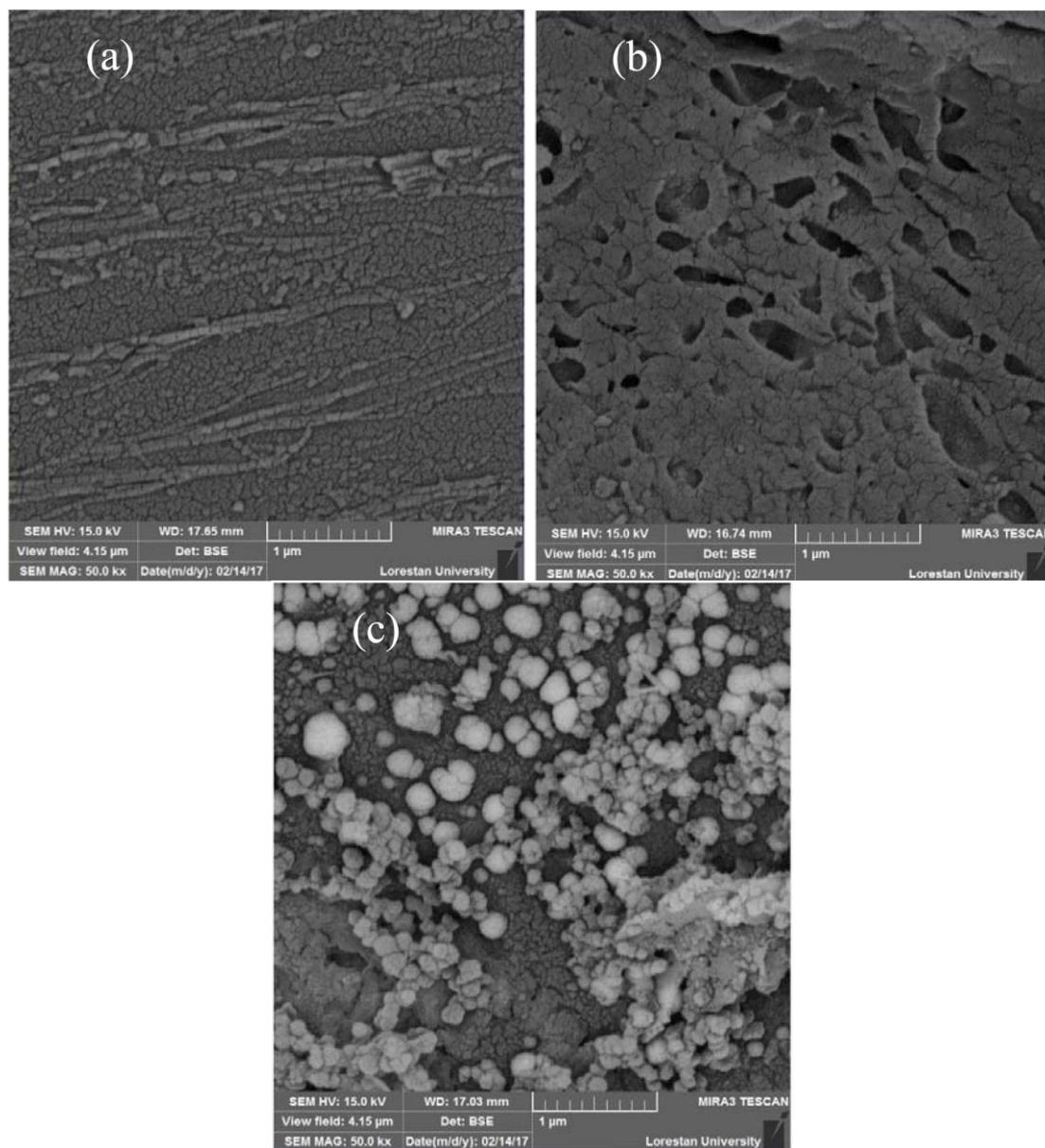
**Figure 2.** The SEM of the P(Ani-co-3ABSA) coating, (a) as synthesized, (b) after templating, and (c) after templating and preconcentrating at  $E = -0.8$  V from  $1.0 \times 10^{-4}$  M  $Pb^{2+}$  solution.
