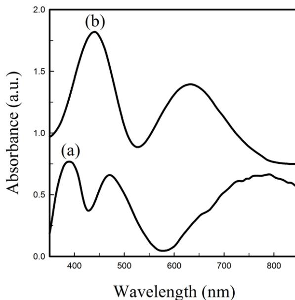
**Figure 1.** The UV spectrum of the copolymeric film on ITO electrodes earlier than (a) and later than (b) the templating process.
