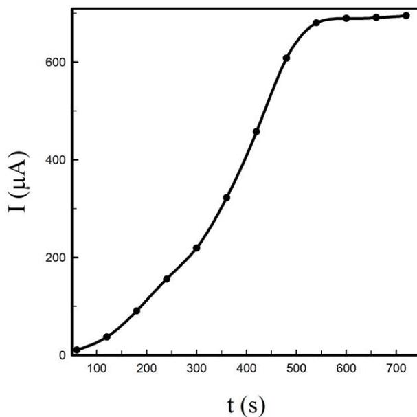
**Figure 6.** The relationship between DP-ASV peak current and pre-concentration time for  $1.0 \times 10^{-4}$  M lead(II) ion.
