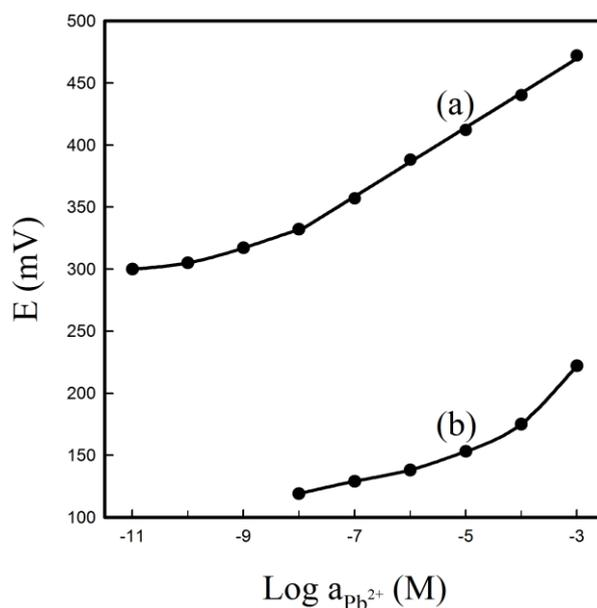
**Figure 9.** Potentiometric working curves for (a) the templated and (b) untemplated P(Ani-co-3ABSA) sensors.
