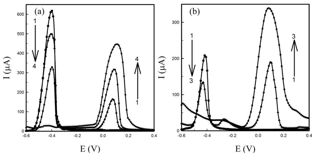
**Figure 8.** The interference effect of  $\text{Cu(II)}$  on the voltammetric measurement of lead (a) by template-modified electrode, (1)  $[\text{Cu}^{2+}]=0$ , (2)  $[\text{Cu}^{2+}]=[\text{Pb}^{2+}]$ , (3)  $[\text{Cu}^{2+}]=10[\text{Pb}^{2+}]$ , (4)  $[\text{Cu}^{2+}]=100[\text{Pb}^{2+}]$ , and (b) by untemplated-modified electrode, (1)  $[\text{Cu}^{2+}]=0$ , (2)  $[\text{Cu}^{2+}]=[\text{Pb}^{2+}]$ , (3)  $[\text{Cu}^{2+}]=10[\text{Pb}^{2+}]$ . For all instances, 0.1 mM lead(II) was used.
