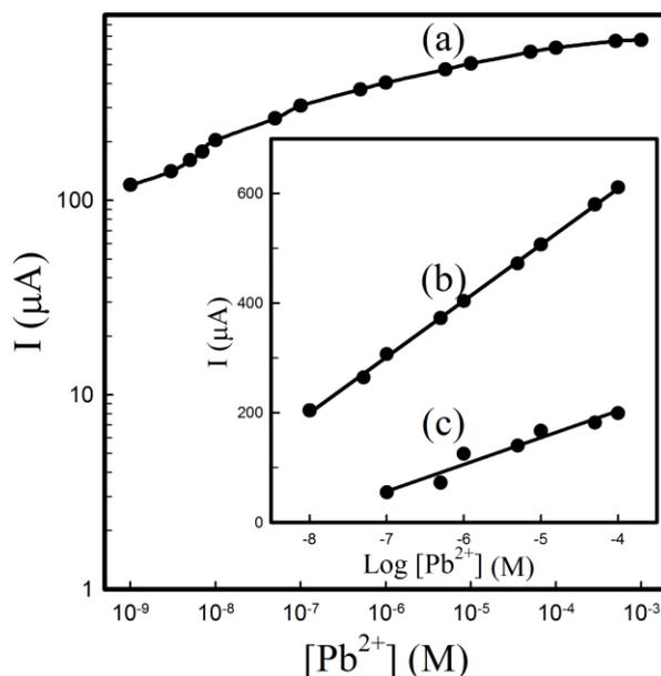
**Figure 7.** The relationship between DP-ASV peak current and lead(II) ion concentration (a). Calibration curves for templated (b) and untemplated (c) electrodes.
