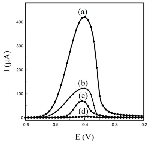
**Figure 4.** DP-ASV of (a) templated-P(Ani-co-3ABSA) coated electrode, (b) untemplated-P(Ani-co-3ABSA) coated electrode, following the pre-concentration of lead, (c) templated-P(Ani-co-3ABSA) coated electrode following the open circuit pre-concentration of lead (d) bare working electrode. For all instances, the molarity of lead(II) was  $1.0 \times 10^{-6}$  M.
