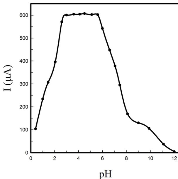
**Figure 5.** Change of the stripping peak intensity with pH of the pre-concentration solution. Electrosynthesis conditions: 0.30 M of 3ABSA and 0.15 M of Ani with potential of 750 mV. Accumulation circumstances:  $\text{Pb}^{2+}$ ,  $1.0 \times 10^{-4}$  M; accumulation potential of  $-800$  mV. DP-ASV circumstances: scanned potential,  $-0.6$  to  $0.4$  V; scanning rate,  $100 \text{ mV s}^{-1}$ ; solution, 0.2 M potassium nitrate with pH = 2.
