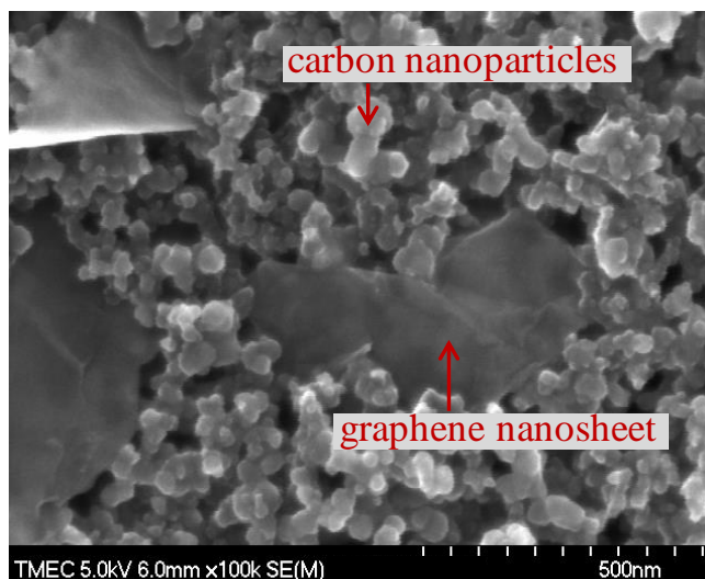
Figure 2. SEM image of graphene modified carbon paste composite
