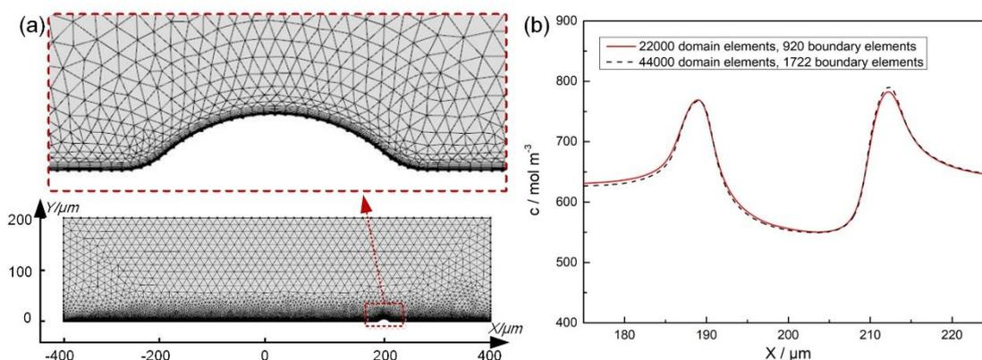
**Figure 4.** Geometric model meshing and validation. (a) Geometric model meshing; (b) mesh validation ( $\varphi_a=5 \text{ V}$ ,  $v_i=4 \text{ m s}^{-1}$ , and  $t=100 \text{ ms}$ ).
