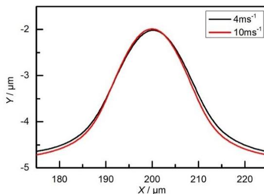
**Figure 11.** Machined anodic shape using flow speeds of 4 and 10  $\text{m s}^{-1}$  ( $\phi_s = 11 \text{ V}$  and  $t = 250 \text{ ms}$ ).
