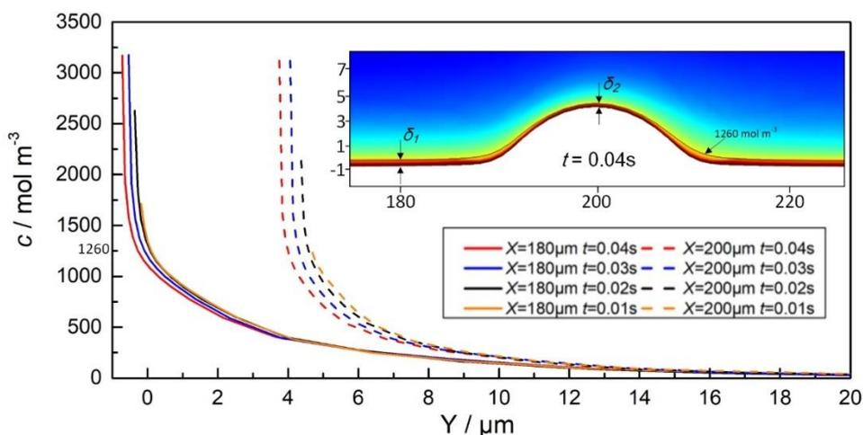
**Figure 7.** Time-dependent change of the distribution of the ion concentration along the  $Y$  axis at 180 and 200  $\mu\text{m}$  ( $\varphi_a = 11 \text{ V}$  and  $v_i = 4 \text{ m s}^{-1}$ ).
