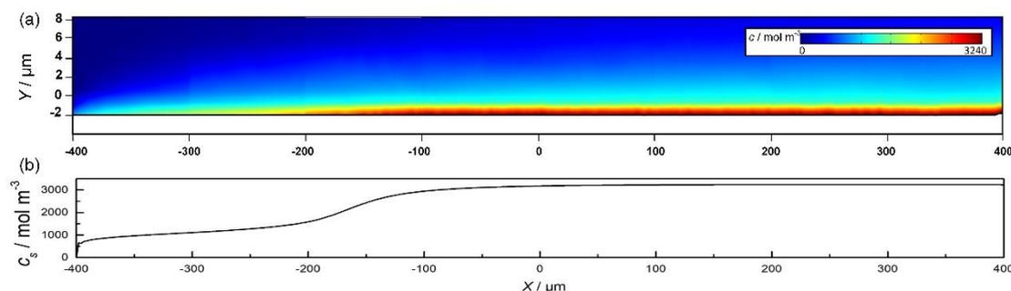
**Figure 5.** Simulation results of the supersaturated film ( $\varphi_a = 11$  V,  $v_i = 4$   $\text{m s}^{-1}$ , and  $t = 100$  ms). (a) Ion concentration near the anode and (b) distribution of interfacial ion concentration along the  $X$  axis.
