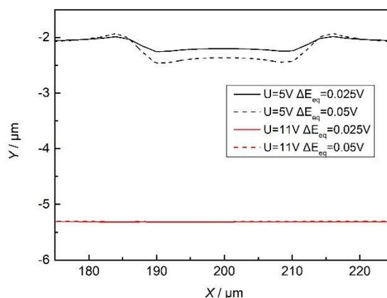
**Figure 13.** Comparison of the anode shape using 5 and 11 V for different microstructures ( $v_i = 4 \text{ m s}^{-1}$  and  $t = 250 \text{ ms}$ ).
