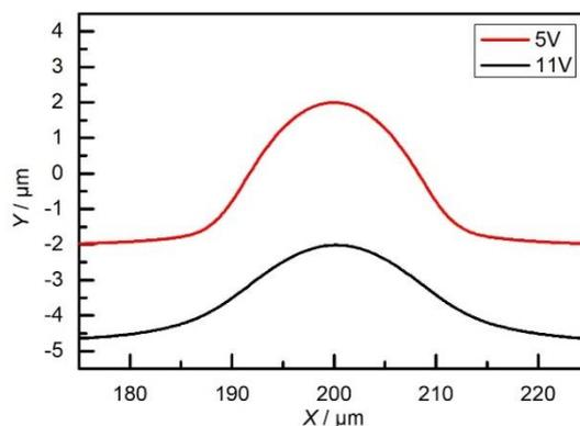
**Figure 9.** Machined anodic shape using 5 and 11 V ( $v_i = 4 \text{ m s}^{-1}$  and  $t = 250 \text{ ms}$ ).
