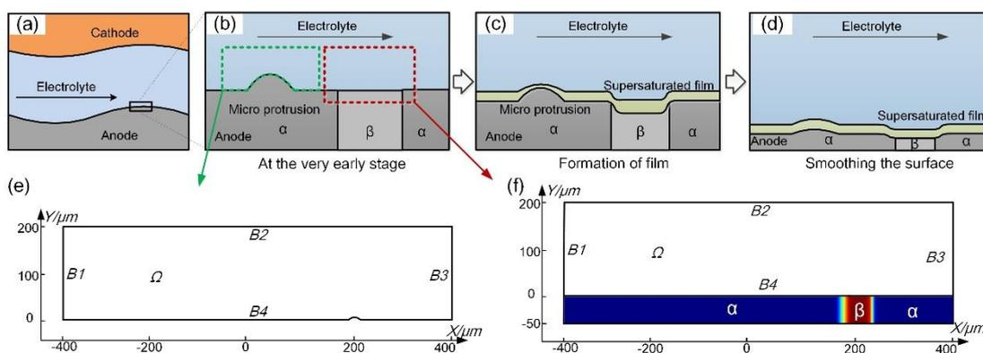
**Figure 2.** Development of the geometric model. (a) Schematic of the ECM inter-electrode gap. (b)–(d) Supersaturated film formation process during ECM. (e) Geometric model for studying parametrical effects. (f) Geometric model for studying the effect of the material's microstructure.
