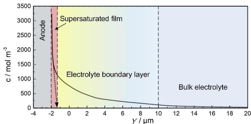
**Figure 6.** Ion concentration distribution along the  $Y$  axis at  $X = 200 \mu\text{m}$  ( $\varphi_a = 11 \text{ V}$ ,  $v_i = 4 \text{ m s}^{-1}$ , and  $t = 100 \text{ ms}$ ).
