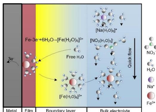
**Figure 3.** Schematic illustration of the electrode reaction kinetics in ECM
