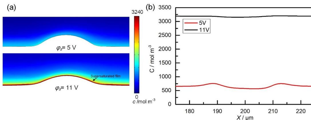
**Figure 8.** Comparison of the distribution of the ion concentration at 5 and 11 V ( $v_i = 4\text{ m s}^{-1}$  and  $t = 250\text{ ms}$ ). (a) Ion concentration distribution near the protrusion. (b) Ion concentration on the anodic surface.
