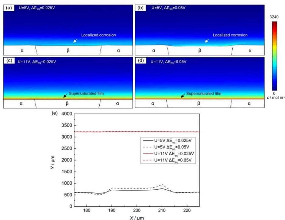
**Figure 12.** Comparison of the ion concentration distribution using applied voltages of 5 and 11 V for different microstructures ( $v_i = 4 \text{ m s}^{-1}$  and  $t = 250 \text{ ms}$ ). (a) Applied potential of 5 V and  $\Delta E_{eq}$  of 0.025 V. (b) Applied potential of 5 V and  $\Delta E_{eq}$  of 0.05 V. (c) Applied potential of 11 V and  $\Delta E_{eq}$  of 0.025 V. (d) Applied potential of 11 V and  $\Delta E_{eq}$  of 0.05 V. (e) Ion concentration on the anodic surface.
