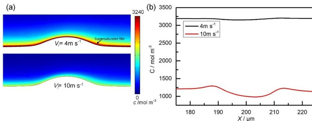
**Figure 10.** Comparison of the distribution of the ion concentration using flow speeds of 4 and 10  $\text{m s}^{-1}$  ( $\phi_a = 11 \text{ V}$  and  $t = 250 \text{ ms}$ ). (a) Ion concentration distribution near the protrusion. (b) Ion concentration on the anodic surface.
