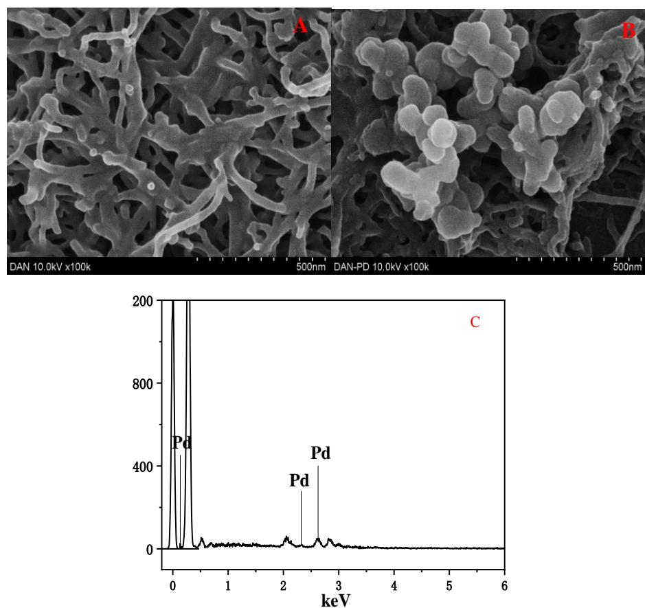
**Figure 1.** SEM of (A) poly(1, 5-DAN)/MWCNTs/GCE and (B) PdNPs-poly(1, 5-DAN)/MWCNTs/GCE; (C) EDX of PdNPs-poly(1, 5-DAN)/MWCNTs/GCE
