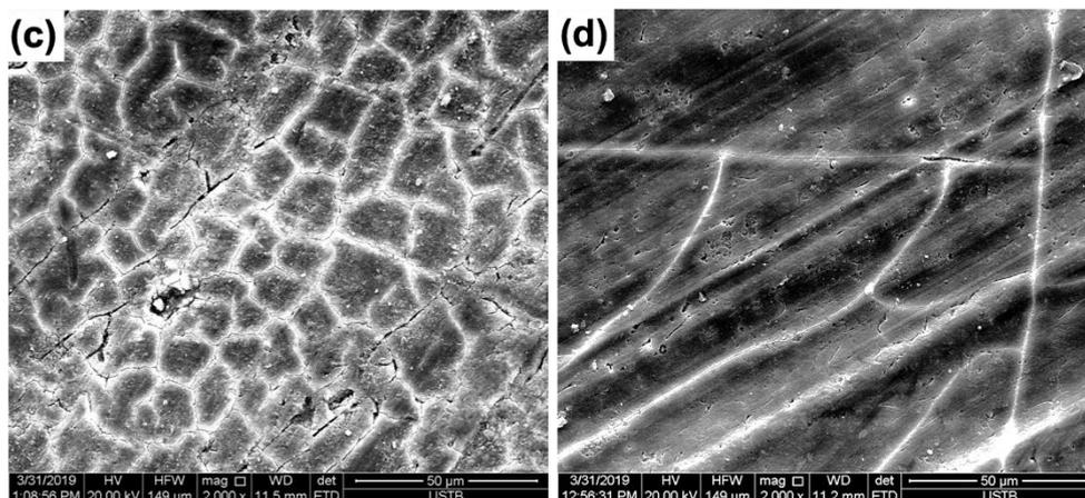
**Figure 2.** Micro corrosion morphology of each sample after removing the rust. (a) and (b) Naked samples exposed for 1 year in Qingdao and Beijing; (c) and (d) anodized samples exposed for 1 year in Qingdao and Beijing
