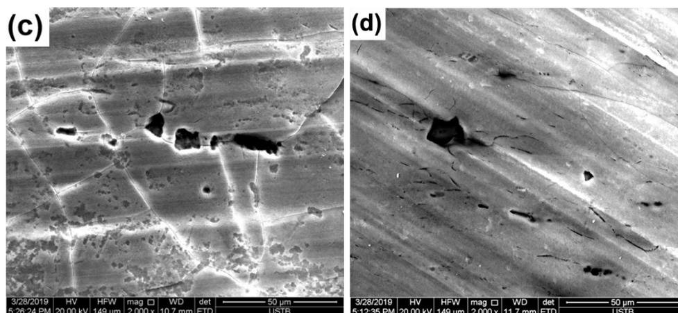
**Figure 4.** Microscopic morphology of samples after removal of the rust layer (a) and (b) Naked samples exposed for 1 year in Qingdao and Beijing Naked samples Initial sample; (c) and (d) Anodized samples exposed for 1 year in Qingdao and Beijing
