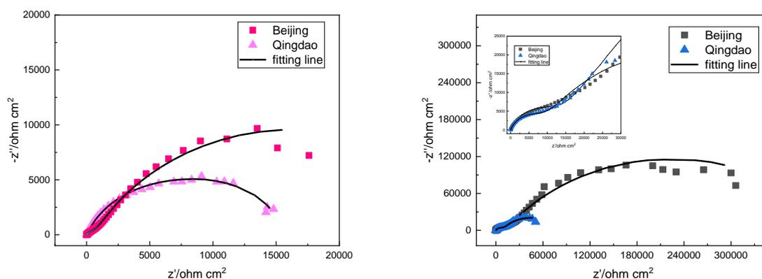
**Figure 8** Nyquist diagram of (a) naked 7B50 samples and (b) anodized samples after one-year exposure in Qingdao and Beijing
