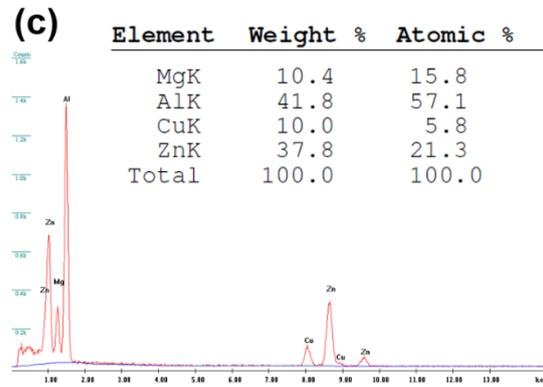
Figure 6. TEM images of (a)-(b) the precipitates along the grain boundary and (c) EDS of the precipitates
