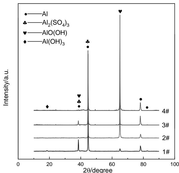
**Figure 3.** XRD patterns of the samples after exposure (1#) naked and (2#) anodized in Qingdao, and (3#) naked and (4#) anodized in Beijing
