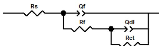
**Figure 9.** Equivalent circle of the exposed 7B50 Al alloy
