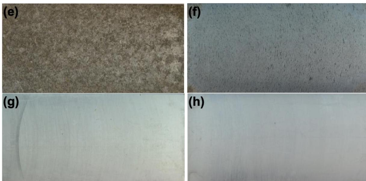
**Figure 1.** Macro corrosion morphology of each sample before removing the rust (a) initial naked sample (b) initial anodized sample; (c) and (d) Naked samples exposed six months in Qingdao and Beijing; (e) and (f) Naked samples exposed a year in Qingdao and Beijing; (g) and (h) anodized samples exposed a year in Qingdao and Beijing
