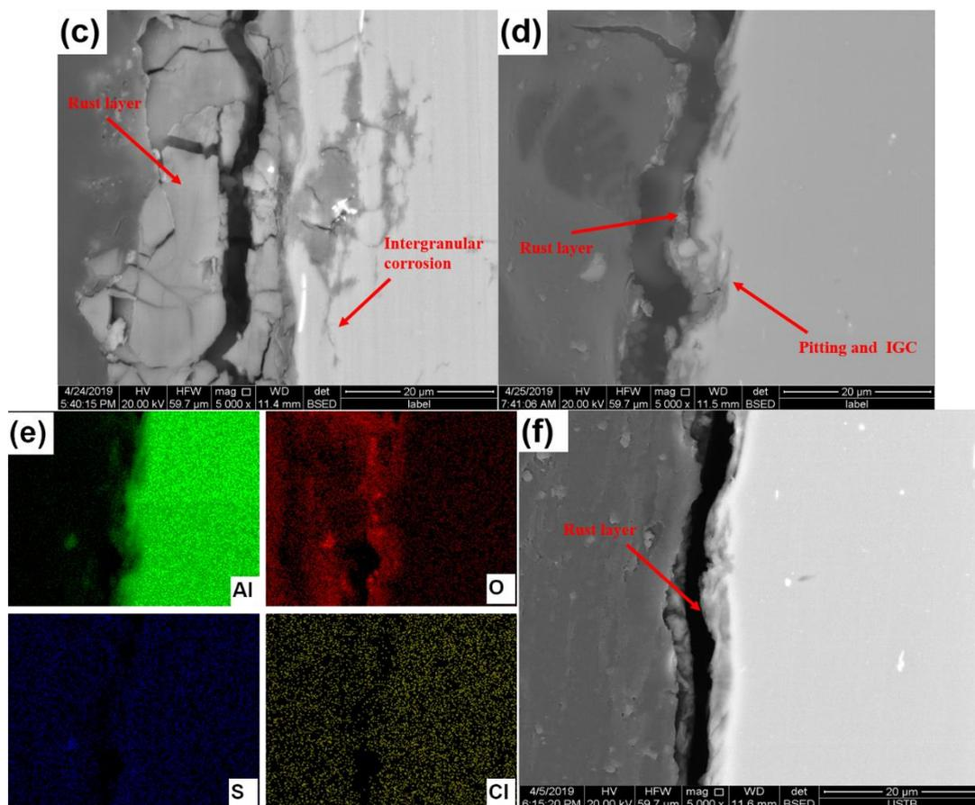
**Figure 5.** Cross-sectional morphologies of the naked samples of after one-year exposure (a) and (c) in Qingdao; (d) and (f) in Beijing and the distribution of elements of (b) the Qingdao sample and (e) the Beijing sample
