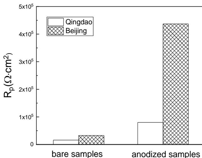
**Figure 10.** Calculated polarization resistance ( $R_p$ ) of the exposed 7B50 Al alloy
