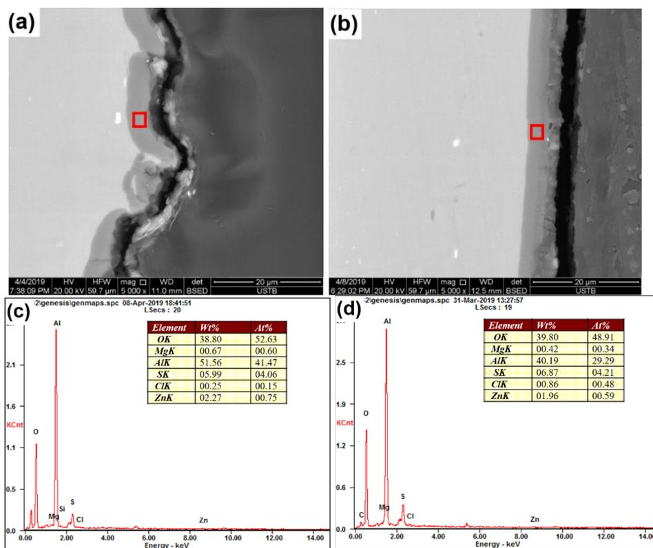
Figure 7. Cross-sectional morphologies and EDS analysis of the anodized samples of (a) and (c) Qingdao; (b) and (d) Beijing
