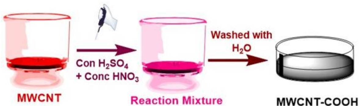
Scheme 1. Functionalization of MWCNT using simple acid treatment procedure.
