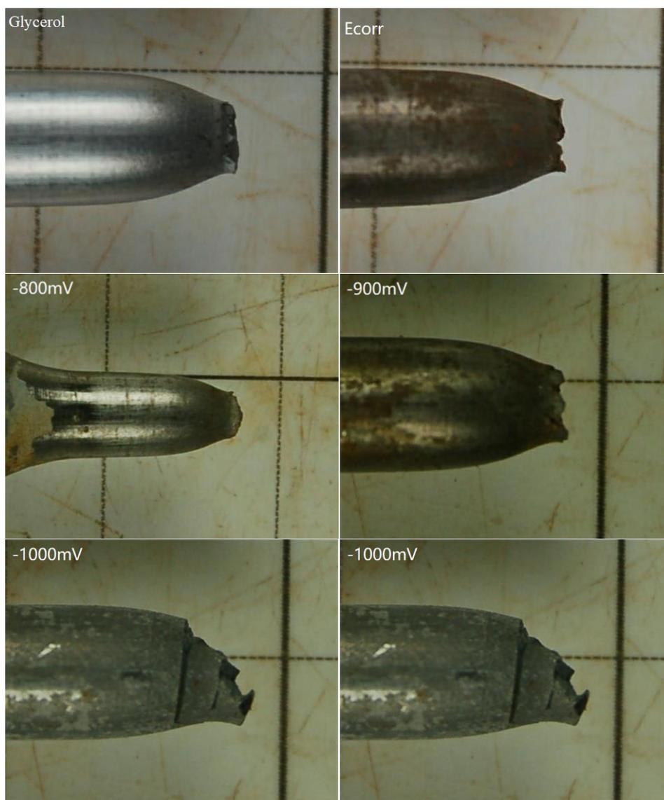
**Figure 9.** Macromorphology of the fracture surface of 10Ni5CrMo steel in glycerol and in seawater at  $E_{corr}$  and applied potential -800mV, -900mV, -1000mV, -1100mV(SCE)
