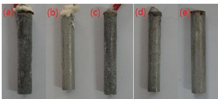
Figure 8. Images of carbon steels in the Cl - -contaminated mortars containing different 0.3% phosphate inhibitors, after 30 days of exposure to a 3.5% NaCl solution, (a) blank mortar and mortar containing (b) ATP, (c) DHP, (d) SPP, (e) COM.
