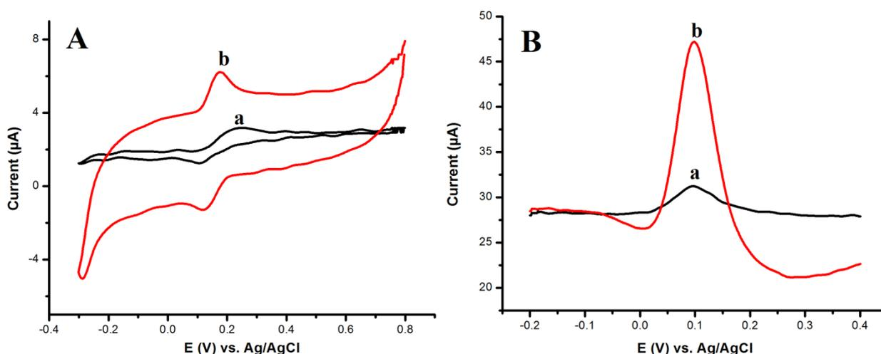
**Figure 3.** The cyclic voltammogram (A) and SW voltammogram (B) of 0.1 mM DOP were recorded at the (a) bare MWCNT and (b) ZLH-SDS-I/MWCNT in 100 mM PBS at pH 8.0.
