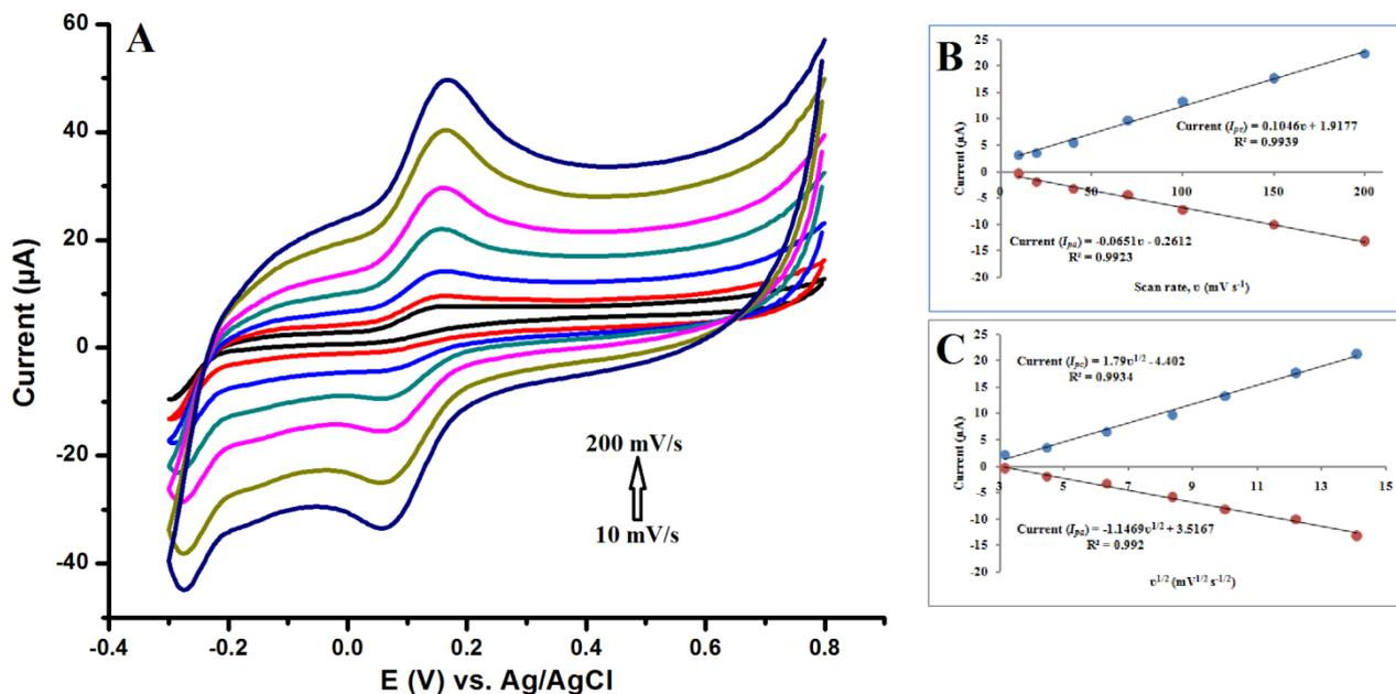
**Figure 5.** CV of 1.0 mM DOP at the ZLH-SDS-I/MWCNT in 100 mM PBS (pH 8.0) at scan rates of 10, 20, 40, 70, 100, 150 and 200  $\text{mV s}^{-1}$  (A), plot of peak currents versus scan rate (B) and the graph of peak currents versus square root of scan rate (C).
