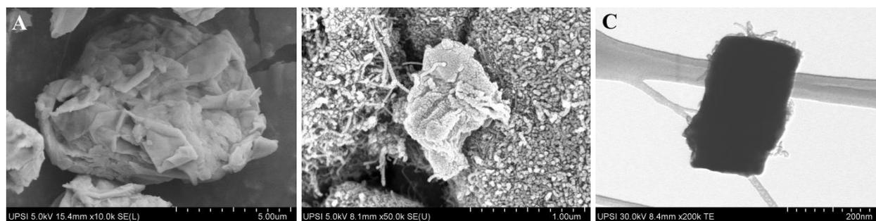
**Figure 1.** SEM images for (A) ZLH-SDS-I; (B) ZLH-SDS-I/MWCNT and (C) TEM image of the ZLH-SDS-I/MWCNT.
