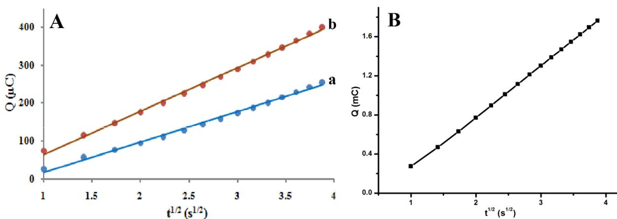
**Figure 4.** Plot of  $Q$  vs.  $t^{1/2}$  on the (A) bare MWCNT (a) and the ZLH-SDS-I/MWCNT (b) towards 4 mM  $[\text{Fe}(\text{CN})_6]^{3-}$  + 100 mM KCl and (B) the ZLH-SDS-I/MWCNT (b) towards 1.0 mM DOP in 100 mM PBS (pH 8.0).
