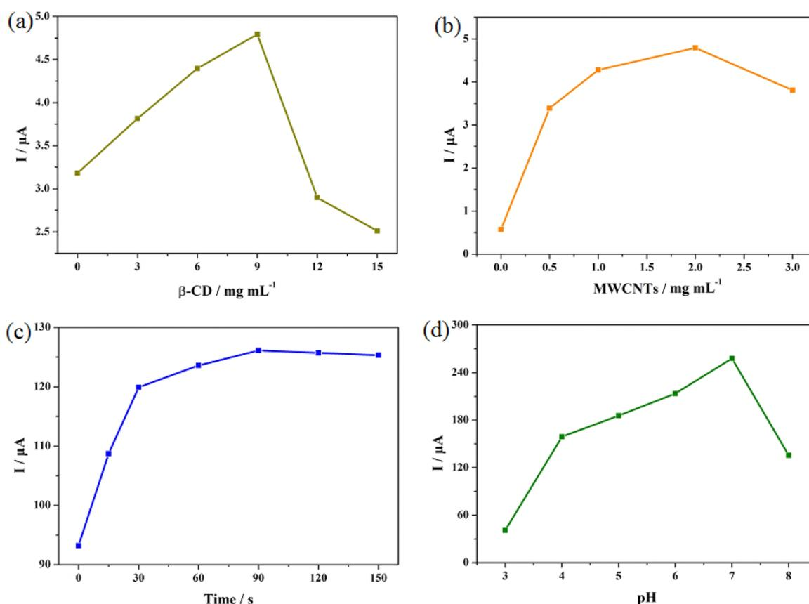
**Figure 5.** Effects of (a)  $\beta$ -CD concentration, (b) MWCNTs concentration, (c) accumulation time, and (d) pH value on the current response were studied by CV or DPV methods, respectively.
