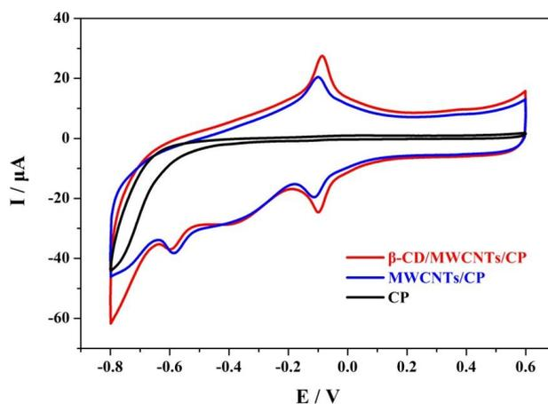
**Figure 4.** CV curves of CP, MWCNTs/CP, and  $\beta$ -CD/MWCNTs/CP in the presence of  $3 \mu\text{g mL}^{-1}$  MP in 0.1 M PBS at pH 7.0 at a scan rate of  $20 \text{ mV s}^{-1}$ .
