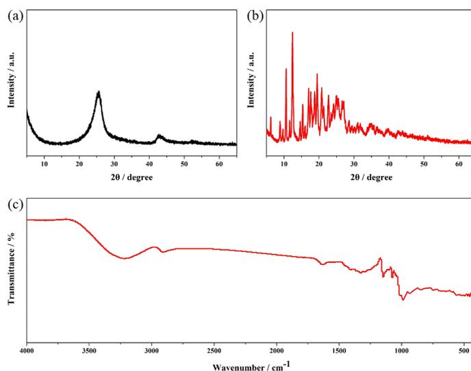
**Figure 1.** XRD patterns of (a) MWCNTs and (b)  $\beta$ -CD/MWCNTs, (c) FTIR spectras of  $\beta$ -CD/MWCNTs.
