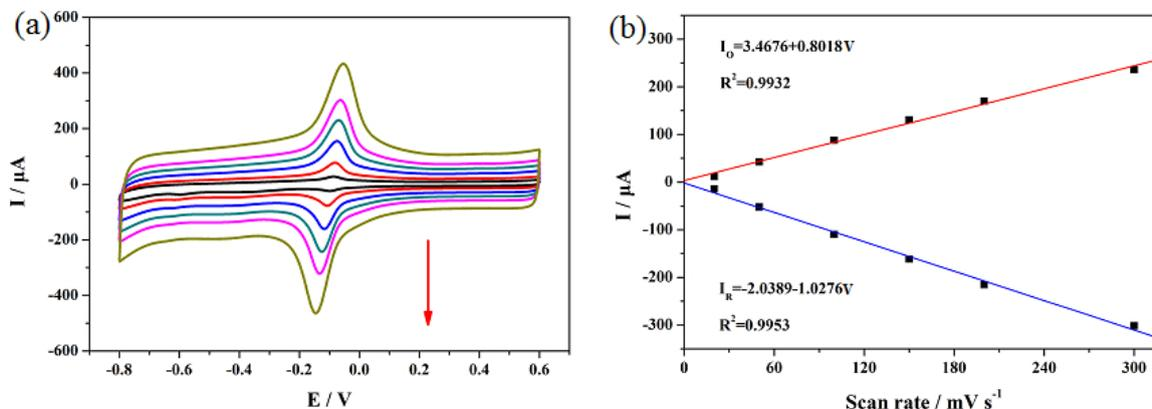
**Figure 6.** (a) CV curves of  $\beta$ -CD/MWCNTs/CP in 0.1 M PBS (PH=7.0) containing  $3 \mu\text{g mL}^{-1}$  MP at a scan rate of 20-300  $\text{mV s}^{-1}$ , (b) the plot of peak current vs. scan rate.
