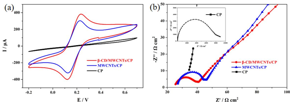
**Figure 3.** (a) CV curves of CP, MWCNTs/CP, and  $\beta$ -CD/MWCNTs/CP in 5 mM  $\text{K}_3[\text{Fe}(\text{CN})_6]/\text{K}_4[\text{Fe}(\text{CN})_6]$  solution containing 0.1 M KCl at a scan rate of  $20 \text{ mV s}^{-1}$ . (b) Nyquist plots of CP, MWCNTs/CP, and  $\beta$ -CD/MWCNTs/CP in 5 mM  $\text{K}_3[\text{Fe}(\text{CN})_6]/\text{K}_4[\text{Fe}(\text{CN})_6]$  solution containing 0.1 M KCl.
