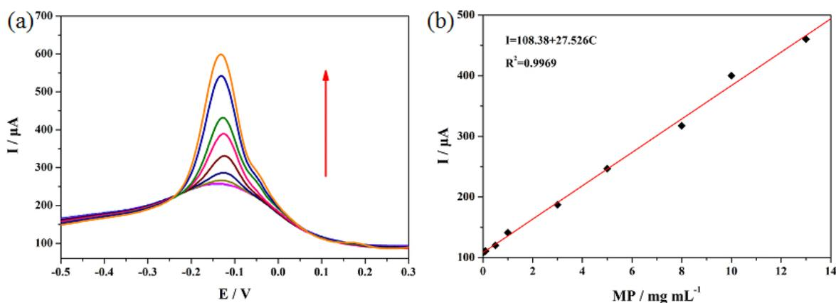
**Figure 7.** (a) DPVs for determination of MP in 0.1 M PBS (PH=7) with  $\beta$ -CD/MWCNTs/CP at MP concentrations ranging from 0.01 to  $13 \mu\text{g mL}^{-1}$  (0.01, 0.05, 0.1, 0.5, 1, 3, 5, 8, 10,  $13 \mu\text{g mL}^{-1}$ ). (b) Linear relationship between oxidation peak current and MP concentration.
