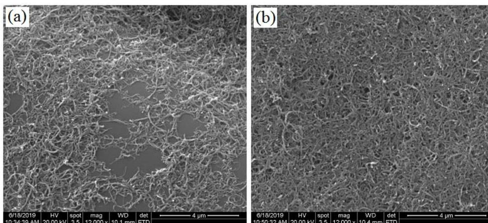
**Figure 2.** SEM images of (a) MWCNTs/CP and (b)  $\beta$ -CD/MWCNTs/CP electrodes.
