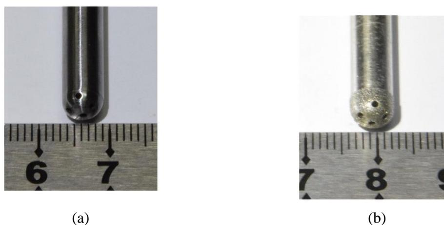
**Figure 5.** Photographs of the columnar electrodes: (a) tool A and (b) tool B.
