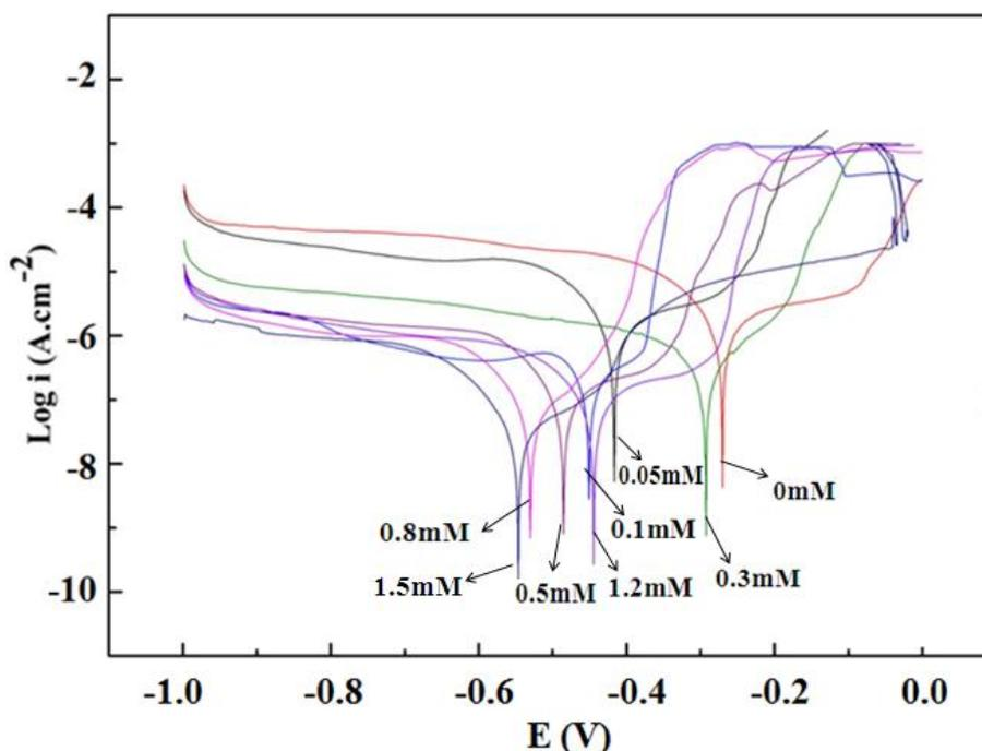
**Figure 3.** Potentiodynamic polarization curves for brass in 0.5 M NaCl in absence and presence of different concentrations of DBN.
