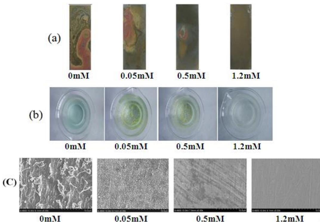
**Figure 6.** Photographs of saline immersion test after 15 days of immersion in 0.5 M NaCl solution. (a) Blank and treated grass (b) Solution after the saline immersion test (c) SEM images of treated grass
