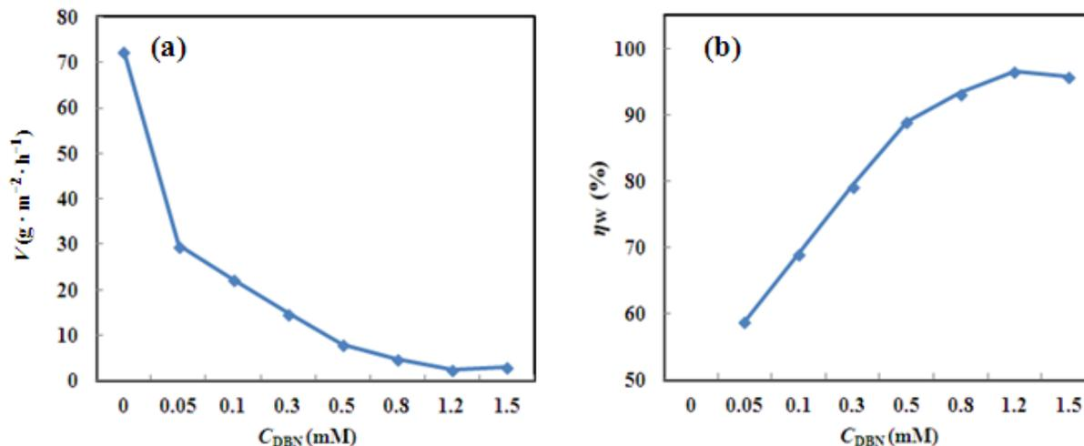
**Figure 2.** Corrosion rates (a) and inhibition efficiency (b) of brass in 0.5 M NaCl with different concentrations of DBN (30 °C).
