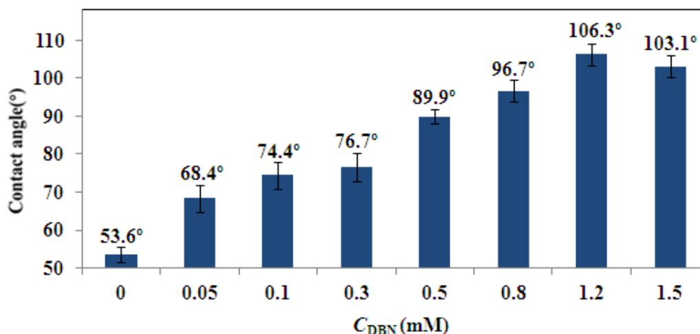
**Figure 5.** Contact angles of brass samples surfaces in 0.5 M NaCl in absence and presence of different concentrations of DBN.
