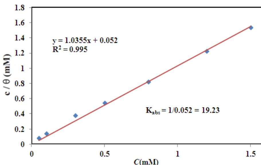
**Figure 4.** Langmuir isotherm adsorption isotherm of DBN in 0.5 M NaCl solution 30 °C.
