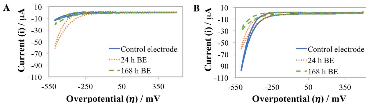
**Figure 6.** Voltammetric analysis of A-Ti materials in biological support media PCNB (a) and AW (b) at 24 h (orange line) and 168 h (green line) after inoculation and CE (blue line).
