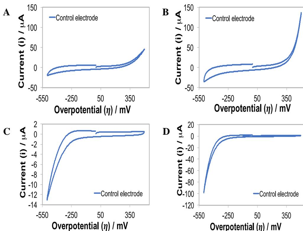
**Figure 2.** Voltammetric analysis of Ti materials in the biological support media PCNB (a) and AW (b) and of A-Ti in the biological support media PCNB (c) and AW (d).
