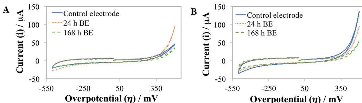
**Figure 4.** Voltammetric analysis of Ti materials in biological support media PCNB (a) and AW (b) at 24 h (orange line) and 168 h (green line) after inoculation and CE (blue line).
