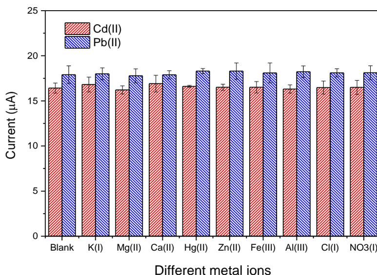
**Figure 8.** The selectivity of the sensing system for 40  $\mu\text{g/L}$  Cd(II) and 40  $\mu\text{g/L}$  Pb(II) over other competing metal ions.
