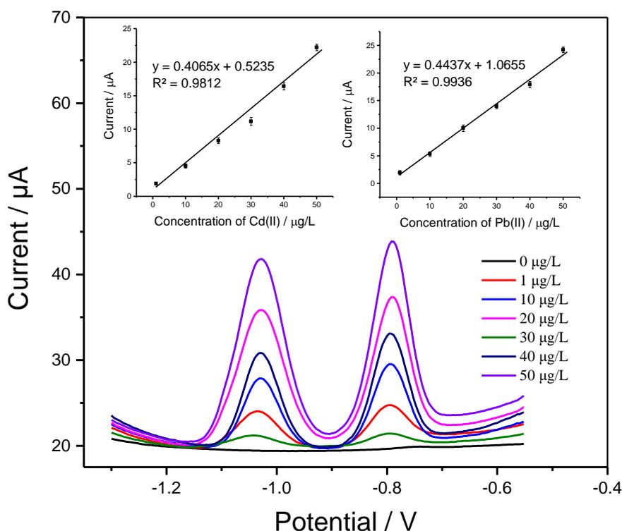
**Figure 7.** SWASV curves of the Bi/G-MWNTs/PBE to detect different Cd(II) and Pb(II) concentrations ranging from 1  $\mu\text{g/L}$  to 50  $\mu\text{g/L}$ ; (A) The calibration curve of Cd(II); (B) The calibration curve of Pb(II)
