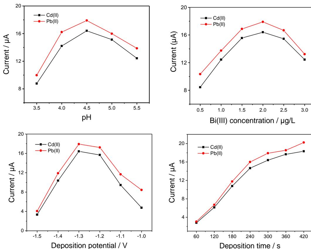
**Figure 6.** The current responses for the determination of 40  $\mu\text{g/L}$  Cd(II) and 40  $\mu\text{g/L}$  Pb(II) in 0.1 mol/L acetate buffer solution affected by (a) bismuth concentration, (b) pH value, (c) deposition potential and (d) deposition time
