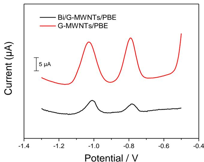
**Figure 5.** The SWV responses of G-MWNTs/PBE before and after electroplated Bi film in 40 µg/L Cd(II) and 40 µg/L Pb(II)
