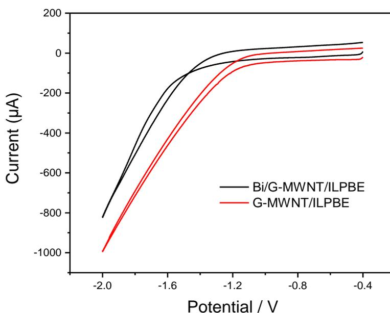
**Figure 4.** Cyclic voltammograms of G-MWNTs/PBE and Bi/G-MWNTs/PBE in 0.1 mol/L acetate buffer solution with the scan rate 100 mV/s
