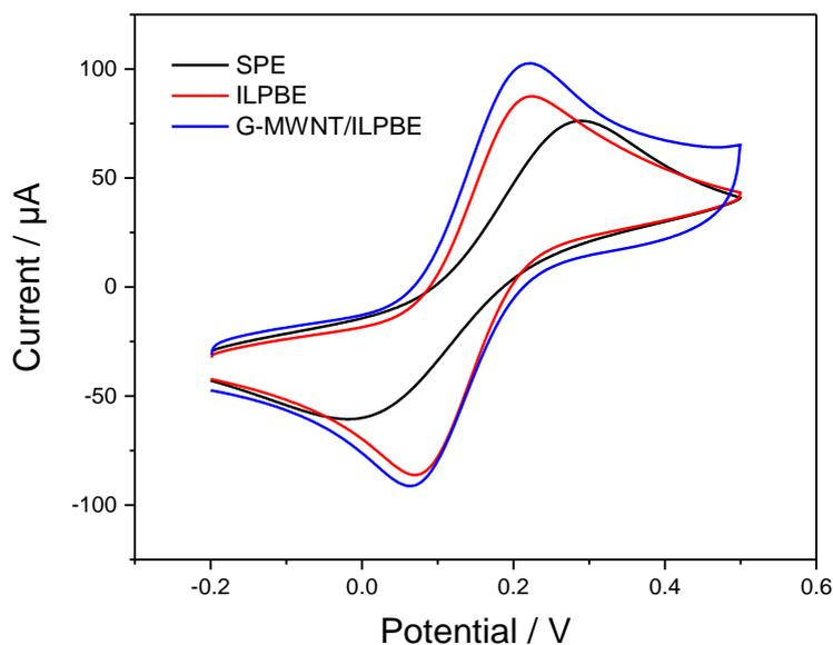
**Figure 2.** CV curves of commercial SPE, PBE, and G-MWNT/PBE in 5 mmol/L  $[\text{Fe}(\text{CN})_6]^{3-/4-}$  containing 0.1 mol/L KCl with the scan rate: 50 mV/s during the potential between -0.2 and 0.5 V.
