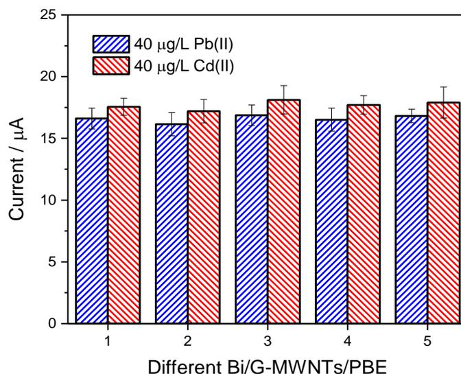
**Figure 9.** The current responses using five different Bi/G-MWNT/PBE for 40  $\mu\text{g/L}$  Cd(II) and 40  $\mu\text{g/L}$  Pb(II).
