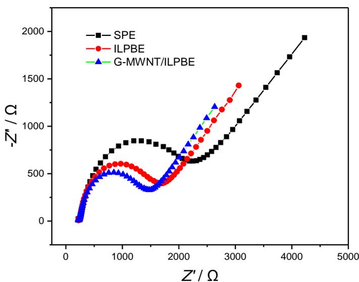
**Figure 3.** Electrochemical impedance spectra of commercial SPE, PBE and G-MWNT/PBE with the frequencies from 1 to  $10^5$  Hz in 5 mmol/L  $[\text{Fe}(\text{CN})_6]^{3-/4-}$  and 0.1 mol/L KCl
