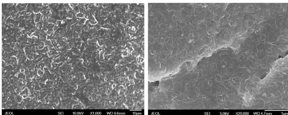
**Figure 1.** SEM images of PBE(a) and G-MWNT/PBE (b).
