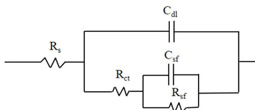
**Figure 10.** Equivalent circuit model used in the fitting of the impedance data
