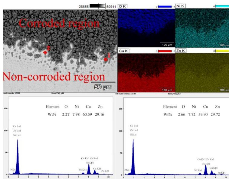
**Figure 3.** SEM mappings and SEM-EDS analysis of the Cu-Zn-Ni alloy scraps in 45 g L<sup>-1</sup> CuSO<sub>4</sub> solutions containing 160 g L<sup>-1</sup> H<sub>2</sub>SO<sub>4</sub> at passive region at 25±1 °C
