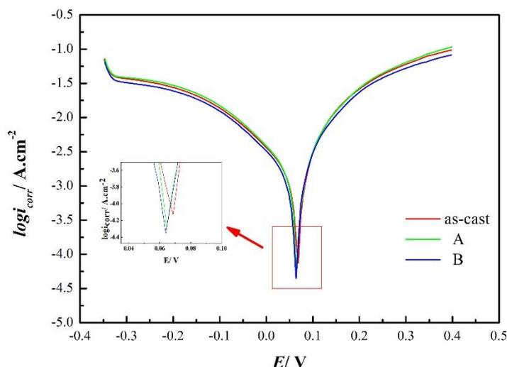
**Figure 8.** Potentiodynamic polarization curves for Cu-Zn-Ni alloy scraps treated in conditions of as-cast, A and B in  $45 \text{ g L}^{-1}$   $\text{CuSO}_4$  solutions containing  $160 \text{ g L}^{-1}$   $\text{H}_2\text{SO}_4$  at scan rate  $5 \text{ mV s}^{-1}$  and  $25 \pm 1 \text{ }^\circ\text{C}$
