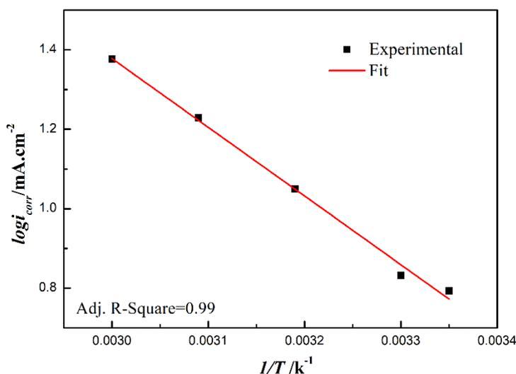
**Figure 5.** Arrhenius plot for Cu-Zn-Ni alloy scraps in  $45 \text{ g L}^{-1} \text{ CuSO}_4$  solutions containing  $160 \text{ g L}^{-1} \text{ H}_2\text{SO}_4$
