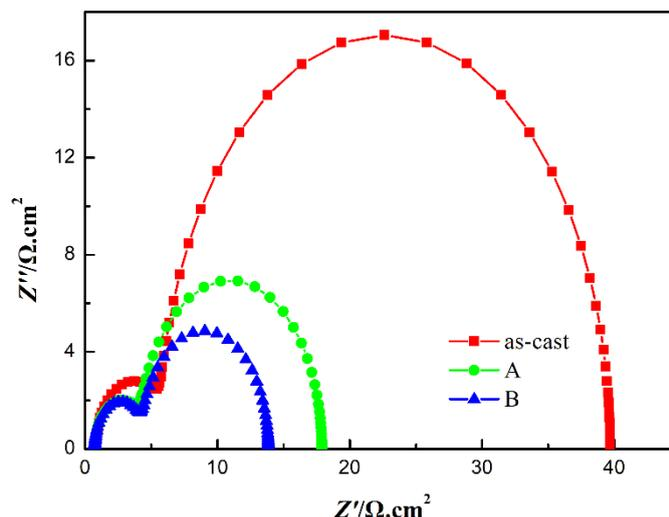
**Figure 9.** Nyquist plot for Cu-Zn-Ni alloy scraps treated in conditions of as-cast, A and B in 45 g L<sup>-1</sup> CuSO<sub>4</sub> solutions containing 160 g L<sup>-1</sup> H<sub>2</sub>SO<sub>4</sub> at 25±1 °C
