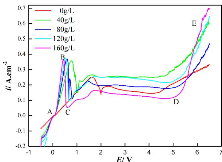
**Figure 2.** Potentiodynamic anode polarization curves for Cu-Zn-Ni alloy scraps in 45 g L<sup>-1</sup> CuSO<sub>4</sub> solutions as a function of sulfuric acid concentration at scan rate 5 mV s<sup>-1</sup> at 25±1 °C
