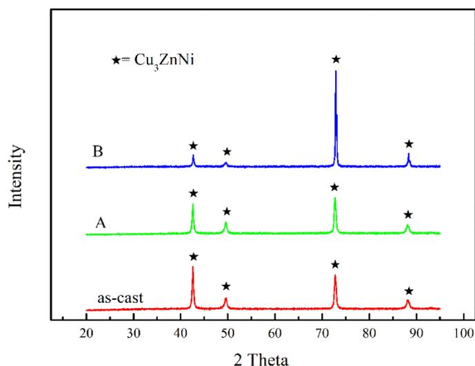
**Figure 7.** X-ray diffraction patterns of Cu-Zn-Ni alloy scraps treated in conditions of as-cast, A and B
