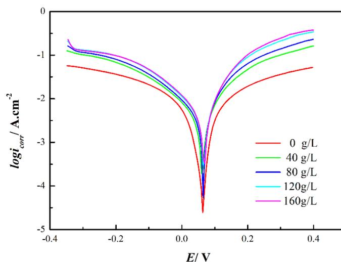
**Figure 1.** Potentiodynamic polarization curves for Cu-Zn-Ni alloy scraps in 45 g  $L^{-1}$   $CuSO_4$  solutions as a function of  $H_2SO_4$  concentration at scan rate 5  $mV s^{-1}$  at  $25 \pm 1$  °C
