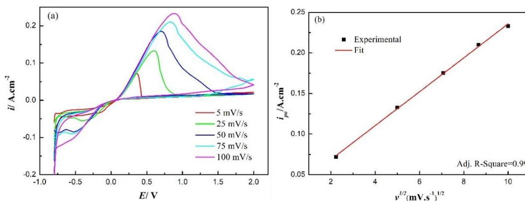
**Figure 4.** Cyclic polarization plots recorded for Cu-Zn-Ni alloy scraps in 45  $\text{g L}^{-1}$   $\text{CuSO}_4$  solutions containing 160  $\text{g L}^{-1}$   $\text{H}_2\text{SO}_4$  with various scan rates at  $25 \pm 1$   $^\circ\text{C}$ : (a) Effect of potential scan rate on cyclic polarization curves; (b) Linear correlation of the anode peak current density against the square root of scan rate
