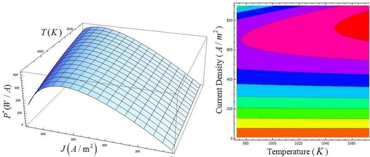
**Figure 2.** the three-dimensional curve of the output power of the coupling system changing with the working current density and temperature.
