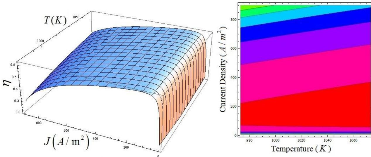
**Figure 1.** three-dimensional curve of the efficiency of the coupling system changing with the working current density and temperature
