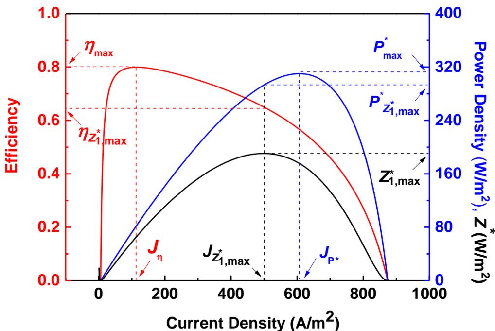
Figure 4. The curves of the efficiency, power density, and  $Z^*$  varying with the current density.
