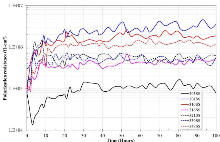
**Figure 8.** Variation in the polarization resistance as a function of time for stainless steels immersed in acetic acid solution (3% v/v) at 40°C.
