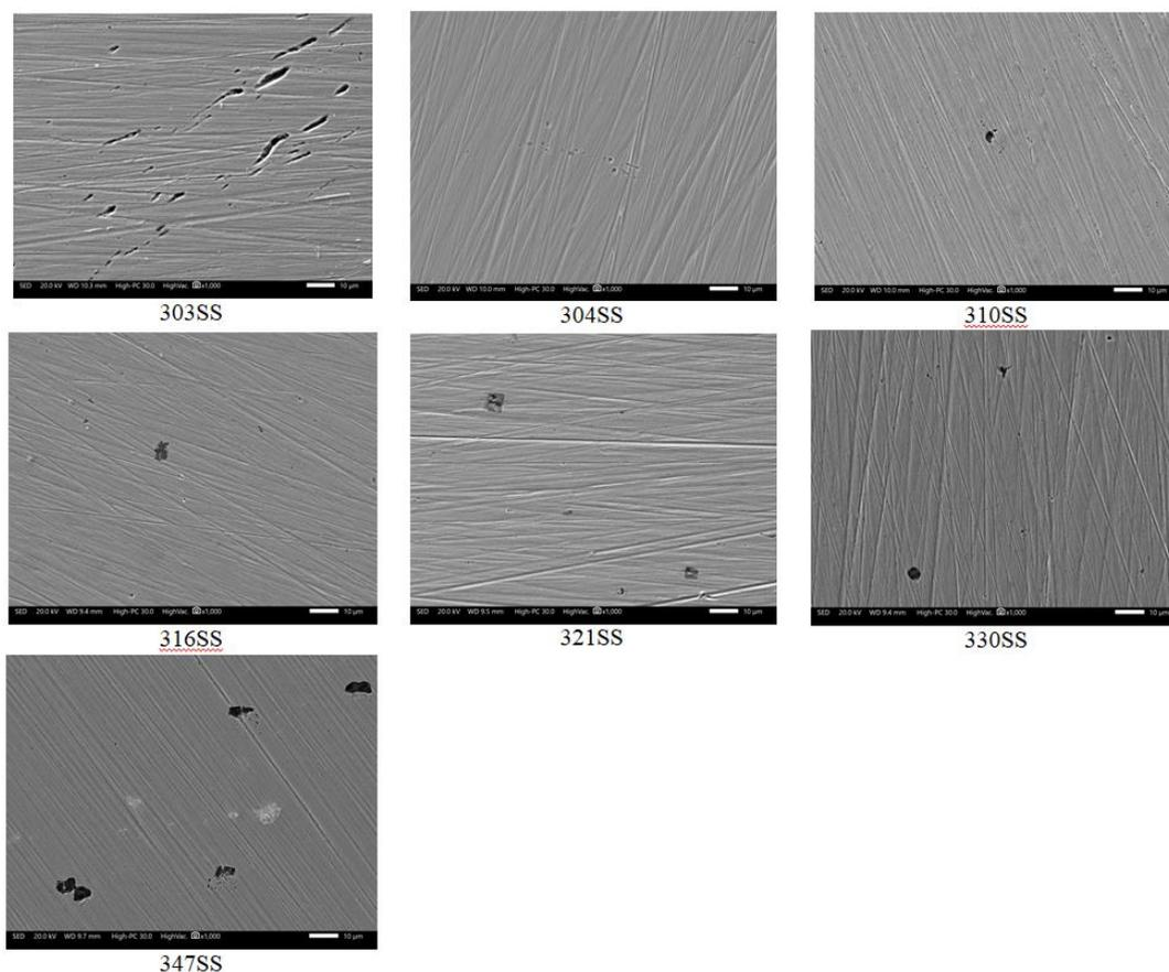
**Figure 15.** Morphological aspects of the austenitic stainless steels after 100 hours of immersion in acetic acid solution at 40°C.
