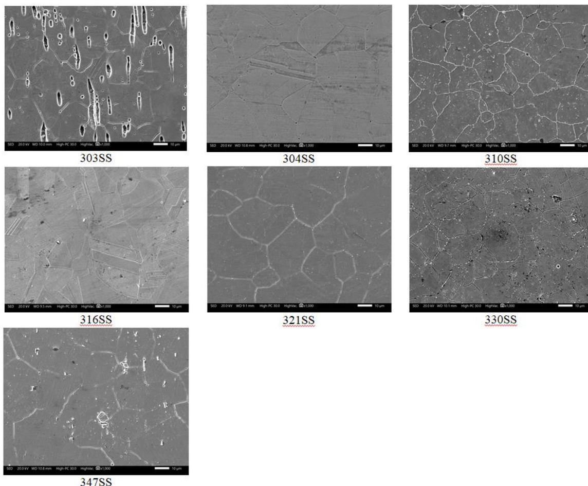
**Figure 1.** Microstructural aspects of different stainless steels.
