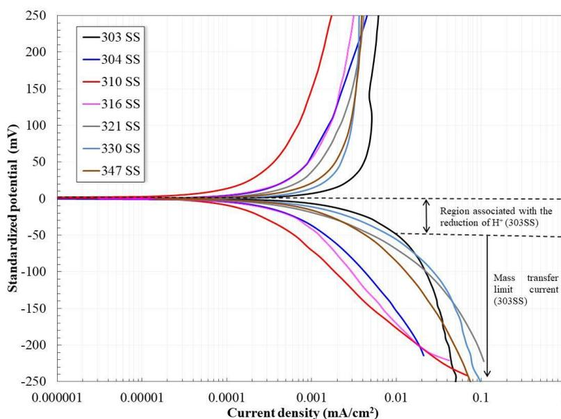
**Figure 3.** Normalized polarization curves and magnification of the Tafel region.
