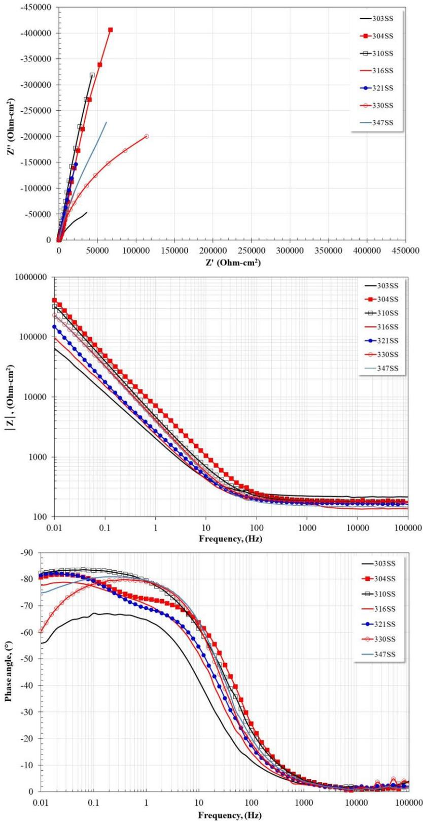
**Figure 9.** Nyquist and Bode diagrams for austenitic stainless steels after 100 hours of immersion in acetic acid solution at 40°C.
