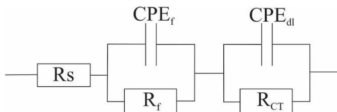
**Figure 11.** Equivalent circuit used for modeling the impedance spectra.
