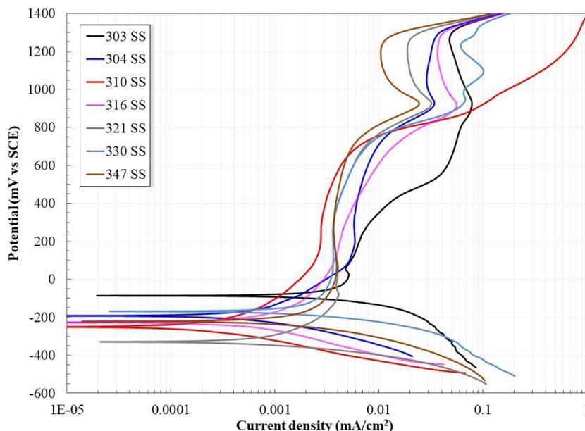
**Figure 2.** Polarization curves for stainless steel in acetic acid solution (3% v/v HAc) at 40°C.
