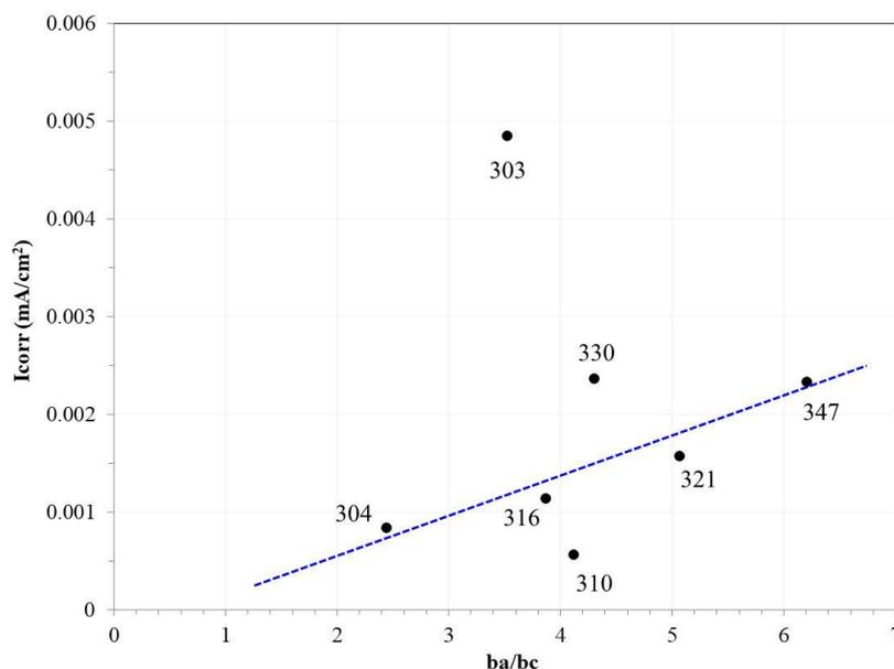
**Figure 6.** Effect of the ba/bc relationship on the  $I_{\text{corr}}$  value of stainless steels.
