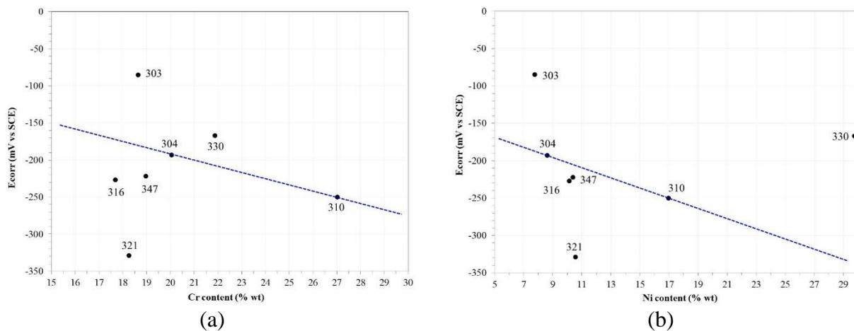
**Figure 4.** Effect of the Cr (a) and Ni (b) content on the corrosion potential of stainless steels.
