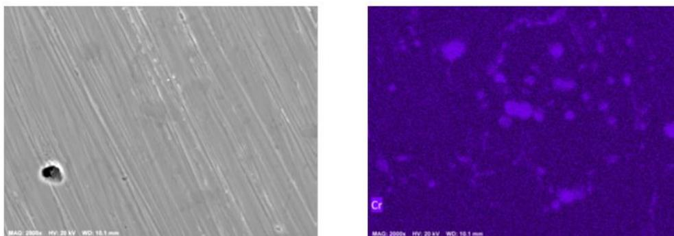
**Figure 16.** Surface aspect and Cr mapping of 310SS after the corrosion test.
