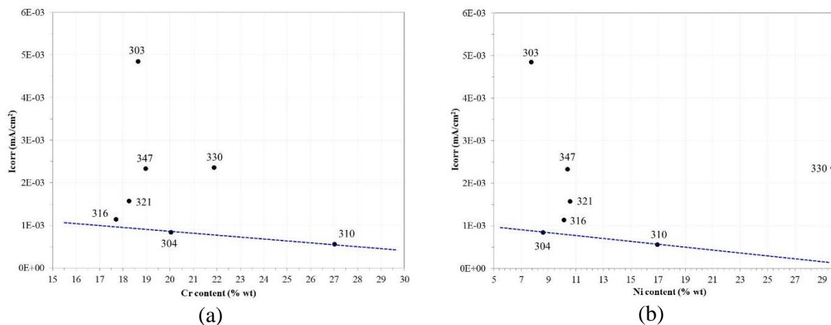
**Figure 5.** Effect of Cr (a) and Ni (b) content on the  $I_{corr}$  values of stainless steels.
