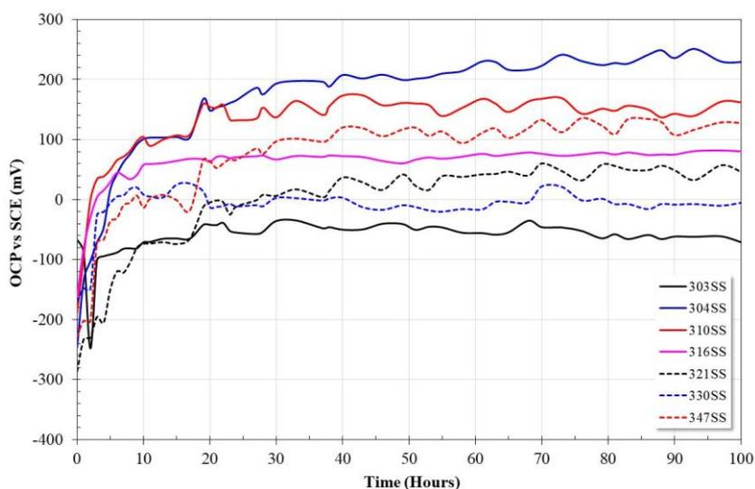
**Figure 7.** Variation of OCP as a function of time for stainless steels immersed in acetic acid solution at 40°C.
