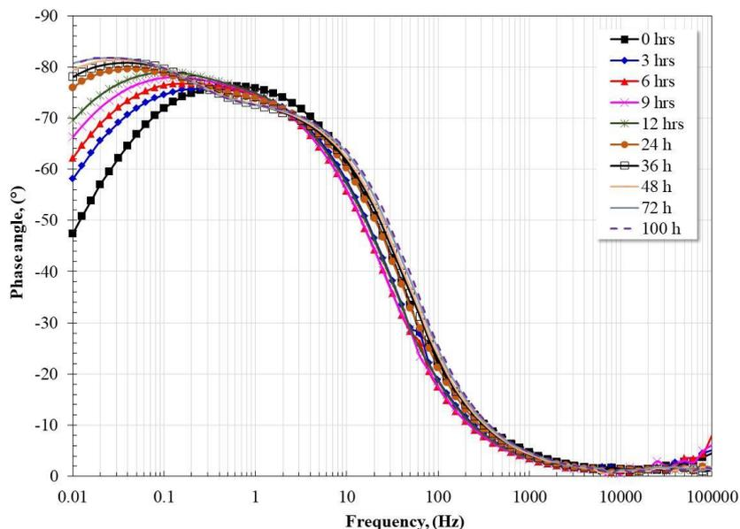
**Figure 10.** Variation of Nyquist and Bode diagrams with respect to immersion time for 304SS in acetic acid solution at 40°C.
