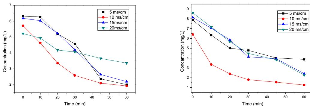
**Figure 4.** Time-dependent change of copper concentration in wastewater for the initial conductivity experiments conducted with the copper (a) and stainless steel (b) cathodes (pH 3; current 0.75 A).
