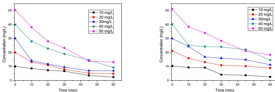
**Figure 5.** Time-dependent change of copper concentration in wastewater for the different initial concentration experiments conducted with the copper (a) and stainless steel (b) cathodes (pH 3; current 0.75 A; conductivity 10mS/cm).
