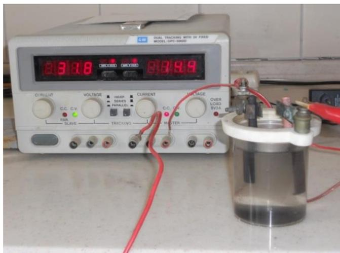
**Figure 1.** Experimental apparatus used in electrodeposition studies.
