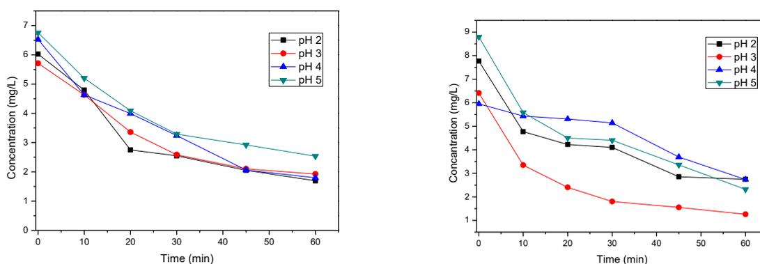
**Figure 3.** Time-dependent change of copper concentration in wastewater for the different initial pH experiments conducted with the copper (a) and stainless steel (b) cathodes (current 0.75 A; conductivity 10 mS/cm).
