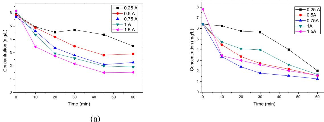
**Figure 2.** Time-dependent change of copper concentration in wastewater for the current experiments conducted with copper (a) and stainless steel (b) cathodes (pH 3; conductivity 10 mS/cm).
