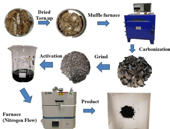
**Figure 1.** Schematic fabrication for the activated carbon.
