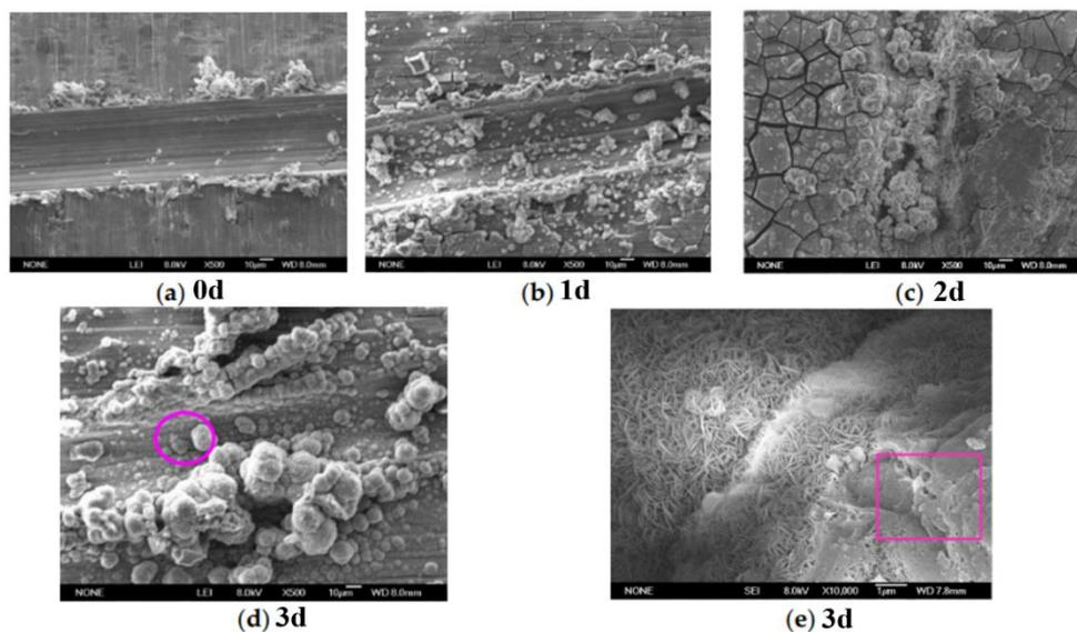
**Figure 2.** Self-healing of vanadia-containing coatings after different immersion times [24] (Creative Commons Attribution License).
