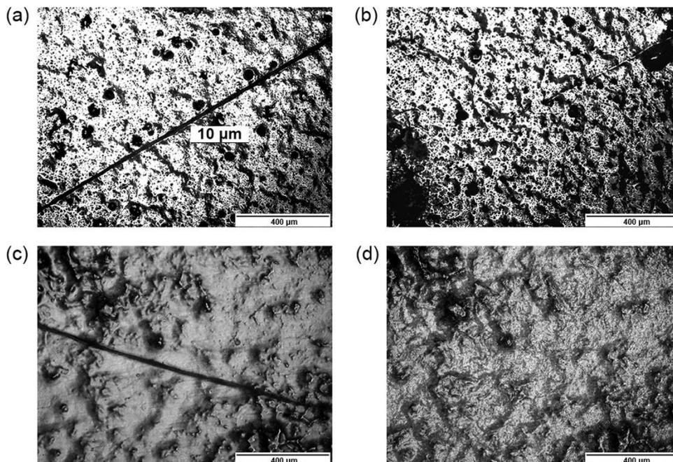
**Figure 6.** Self-healing offered by ceria in a layer-by-layer coating [43] (Reproduced with permission from American Chemical Society).
