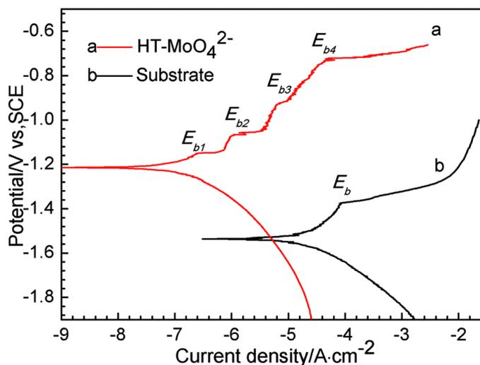
**Figure 9.** Self-healing of a molybdate-intercalated LDH coating investigated with PPT [30] (Reproduced with permission from Royal Society of Chemistry).
