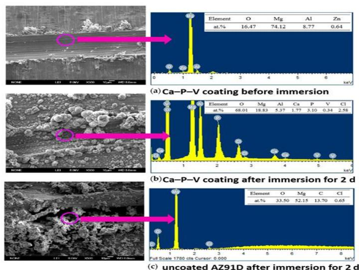
**Figure 7.** Scratch test examined with SEM and EDS [24] (Creative Commons Attribution License).
