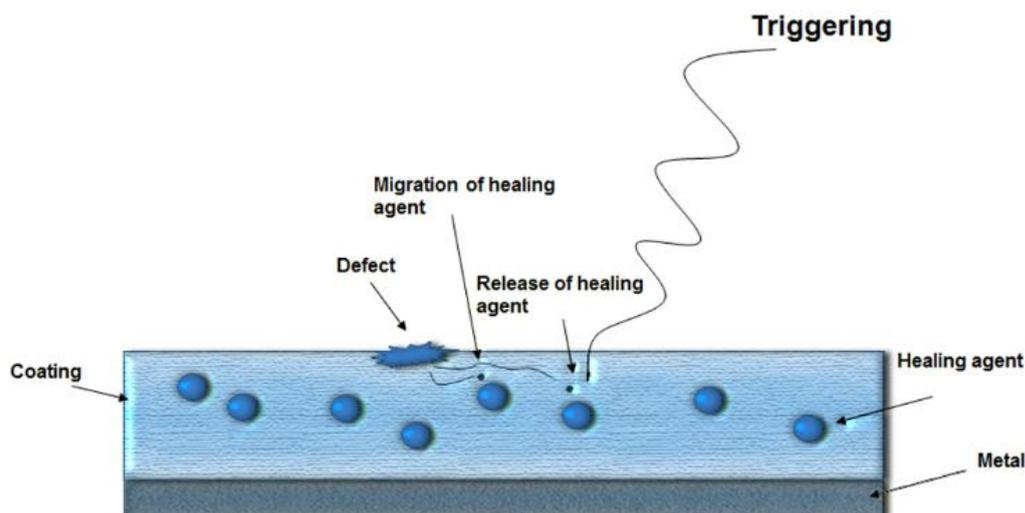
**Figure 1.** Schematic of the self-healing coating mechanism on metallic substrates.
