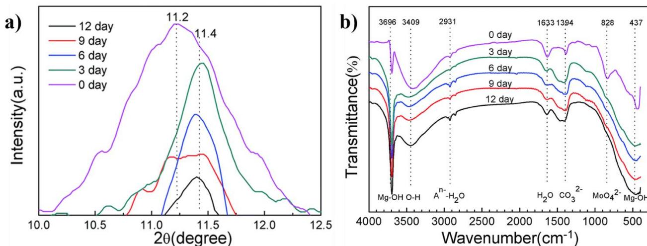
**Figure 8.** The shifting in XRD peaks (a) and band weakening in FTIR (b) of a molybdate-intercalated LDH [30] (Reproduced with permission from Royal Society of Chemistry).
