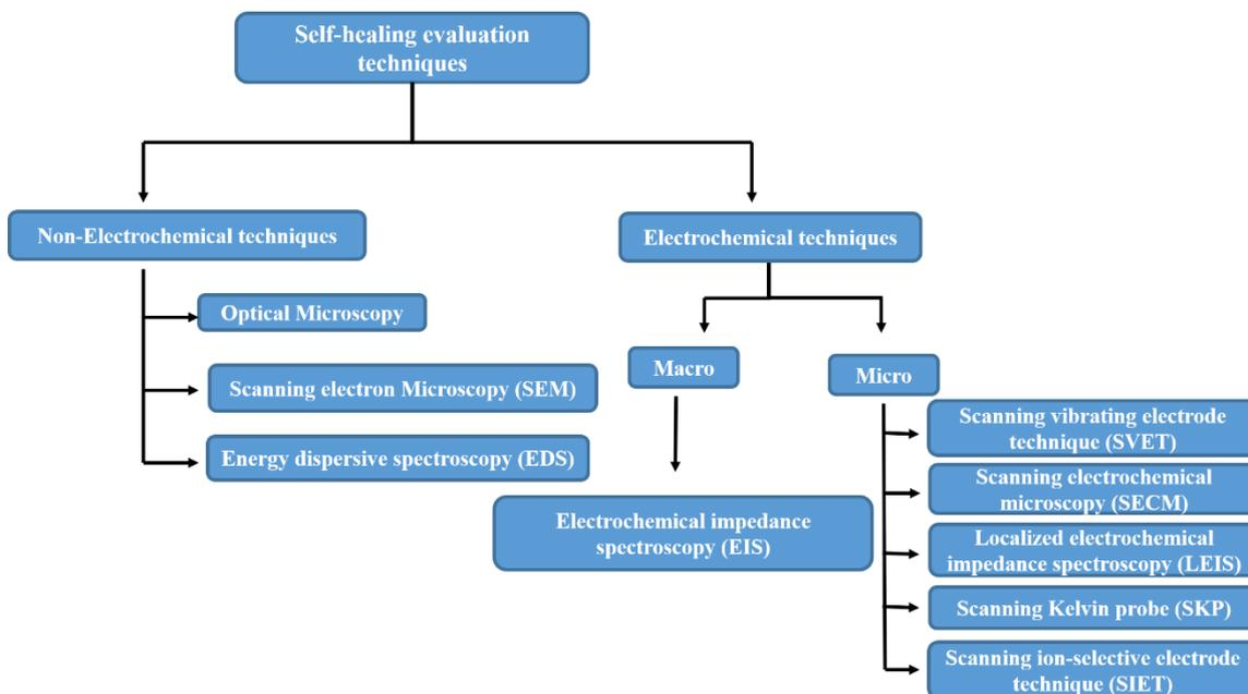
**Figure 5.** Self-healing evaluation techniques used for Mg alloy coatings.
