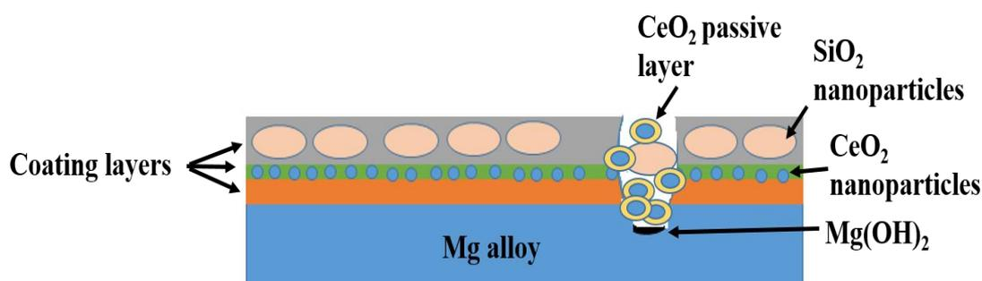
**Figure 3.** Self-healing offered by  $\text{CeO}_2$  nanoparticles.
