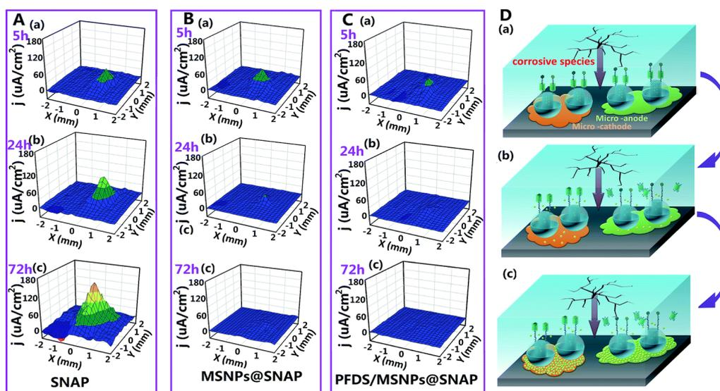
**Figure 10.** SVET studies to understand the healing mechanism of HMAP [39] (Reproduced with permission from Royal Society of Chemistry).
