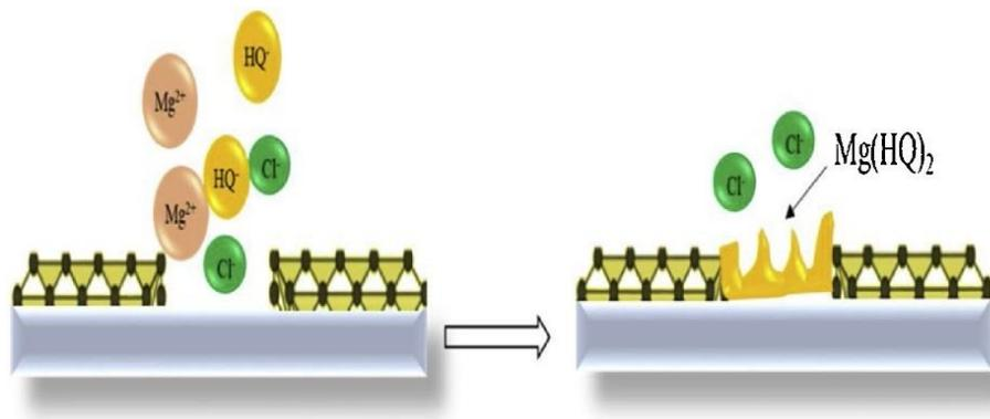
**Figure 4.** Self-healing mechanism offered by 8HQ [28] (Reproduced with permission from Elsevier).
