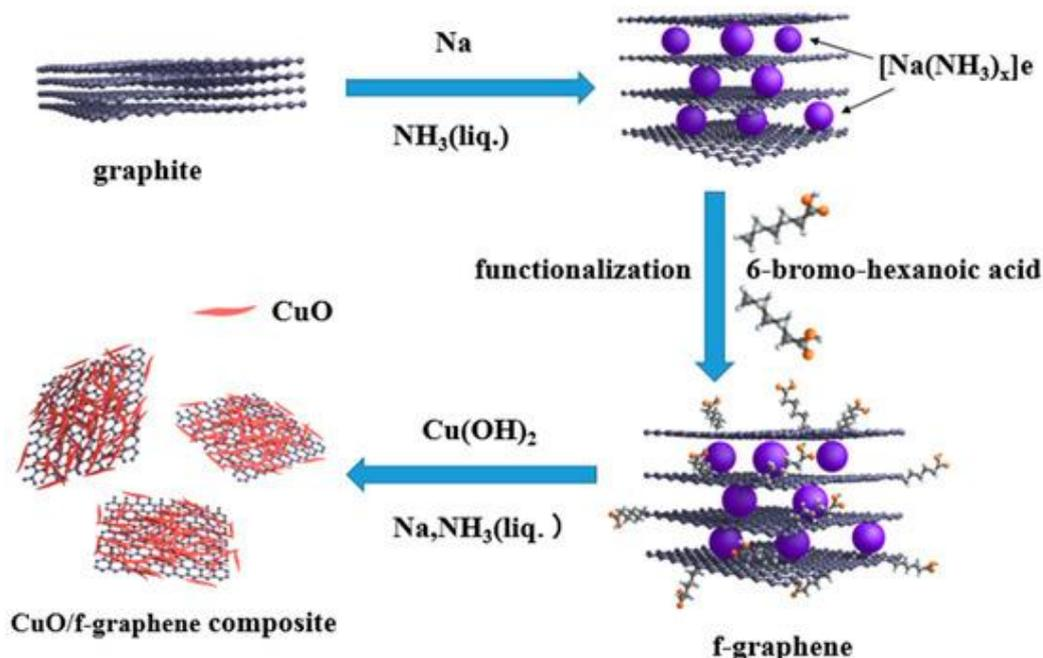
**Figure 1.** Schematic of the synthesis procedure of the CuO/f-graphene composite. Copyright obtained from MDPI [107].
