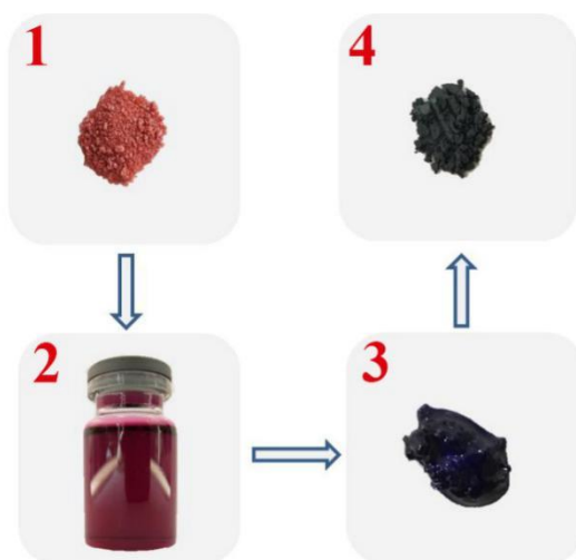
Figure 1. Photos of all materials appearing in the preparation process. Photo 1 was for cobaltous acetate tetrahydrate. Photo 2 was the photo of the suspension solution containing \text{Co}(\text{CH}_3\text{COO})_2 \cdot 4\text{H}_2\text{O} , 1-butyl-3-methylimidazolium bromide, double-distilled water and ethanol. Photo 3 was the photo of the well-dried materials which was a black and viscous substance. Photo 4 was the final material, a black powder.
