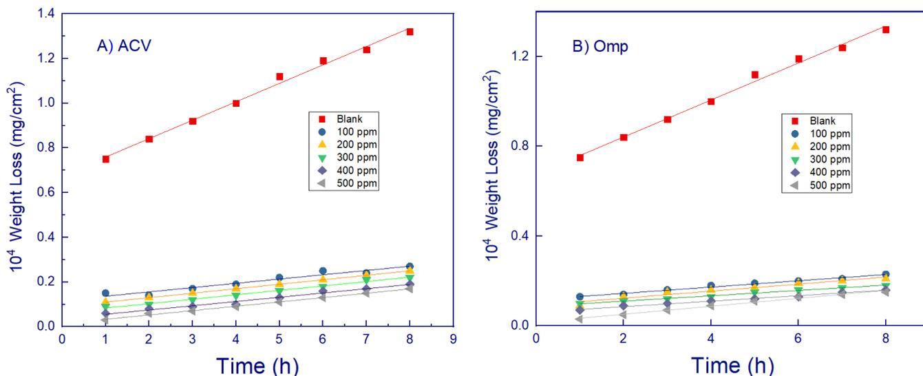
**Figure 1.** Weight loss (WL) versus immersion time for the corrosion of Sabcic iron in free 1.0 M HCl solution (blank) and with various concentrations of expired A) ACV and, B) Omp at 25 °C.
