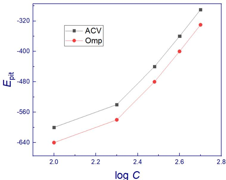
**Figure 8.** The relationship between  $E_{\text{pit}}$  and  $\log C$  of the investigated drugs for the corrosion of Sabcic iron in 1.0 M HCl + 0.5 M NaCl solution in the presence of ACV and OMP.
