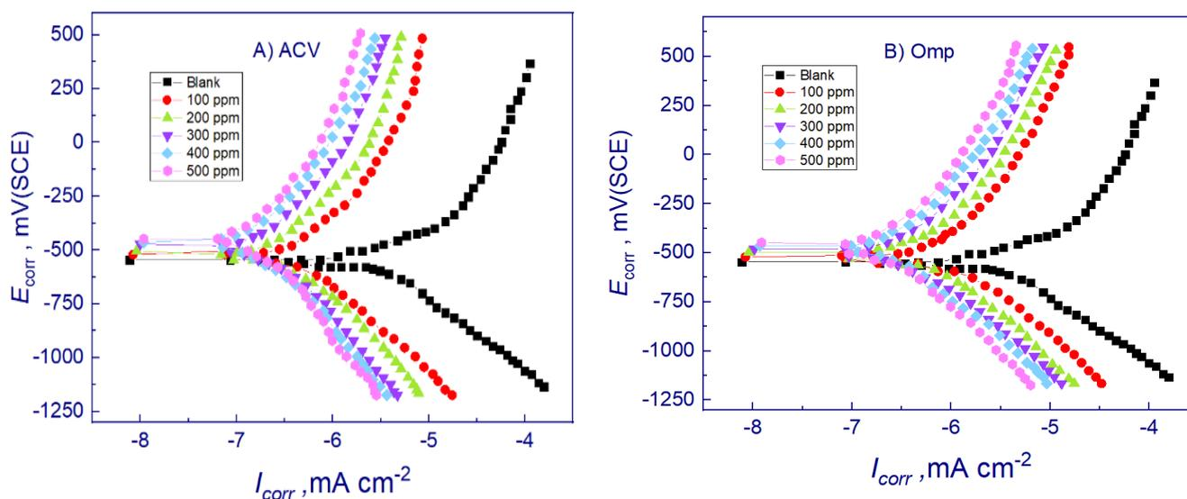
**Figure 5.** GAP polarization curves for the corrosion of Sabcic iron in 1.0 M HCl solution and containing different concentrations of the expired drugs: A) ACV and B) OMP
