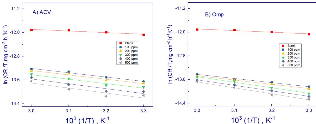
**Figure 3.** Plots of  $\ln (CR/T)$  versus  $1/T$  for the corrosion of Sabic iron in 1.0 M HCl solution and containing some concentrations of the expired drugs: A) ACV and B) OMP.
