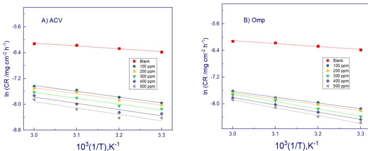
**Figure 2.** Plots of log CR versus 1/T for the corrosion of Sabcic iron in 1.0 M HCl solution and including various concentrations of drugs: A) ACV and B) OMP.
