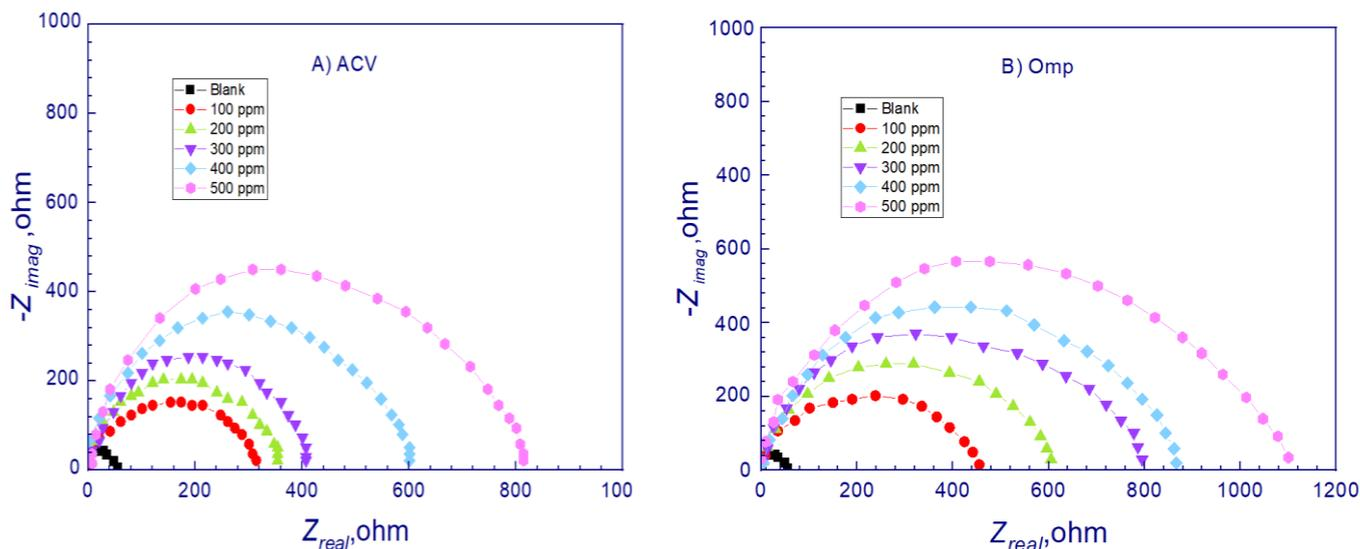
**Figure 6.** Nyquist plots for the corrosion of Sabic iron in 1.0 M HCl solution and including some concentrations of the expired drugs: A) ACV and B) OMP at 25 °C.
