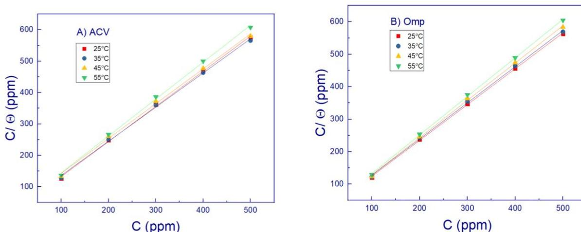
**Figure 4.** The relationship between  $C/\theta$  versus  $C$  for the adsorption of ACV and OMP drugs on Sabcic iron surface in 1.0 M HCl solution at different temperatures (Langmuir isotherm)
