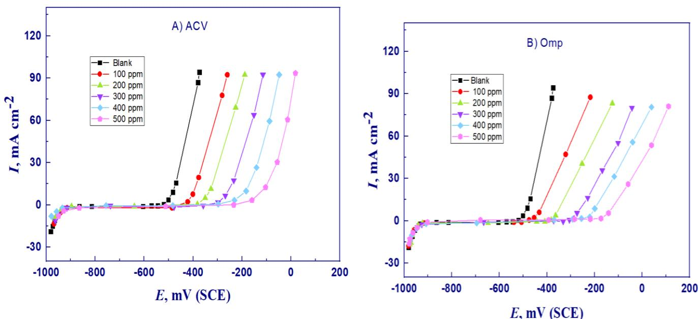
**Figure 7.** PAP curves of Sabic iron corrosion in 1.0 M HCl + 0.5 M NaCl solution and including various concentrations of the expired drugs: A) ACV and B) OMP, at scan rate 1.0 mV s<sup>-1</sup>.
