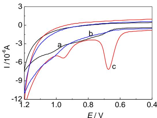
**Figure 3.** CV curves of guanine and adenine with the different electrodes in 0.1 M PBS (pH 7.0) and a scan rate of 100 mV/s: a- bare GCE; b- RGO/GCE; and c- PDA/RGO/GCE.
