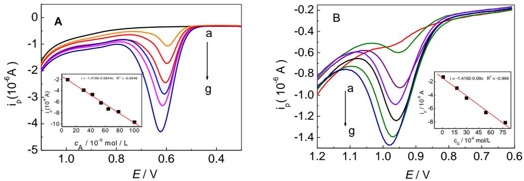
**Figure 7.** DPV curves of the different concentrations of guanine (A) and adenine (B) with PDA/RGO/GCE in 0.1 mol/L PBS (pH 7.0). The inset shows the oxidation peak current of guanine and adenine vs. concentration.
