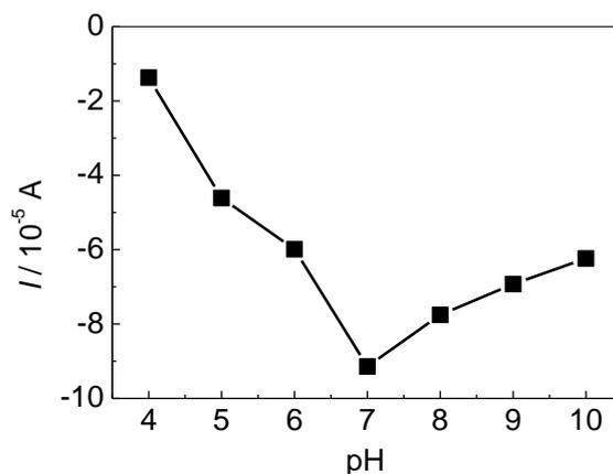
**Figure 4.** Relationship of the oxidation peak current of PDA/RGO/GCE at various pH values.
