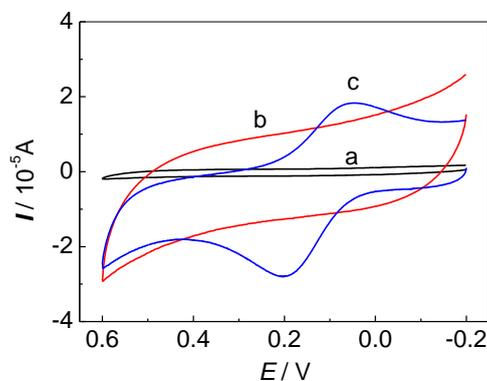
**Figure 1.** CV curves of the different electrodes in 0.1 M PBS (pH 7.0) with a scan rate of 50 mV/s: a- bare GCE; b- RGO/GCE; and c- PDA/RGO/GCE.
