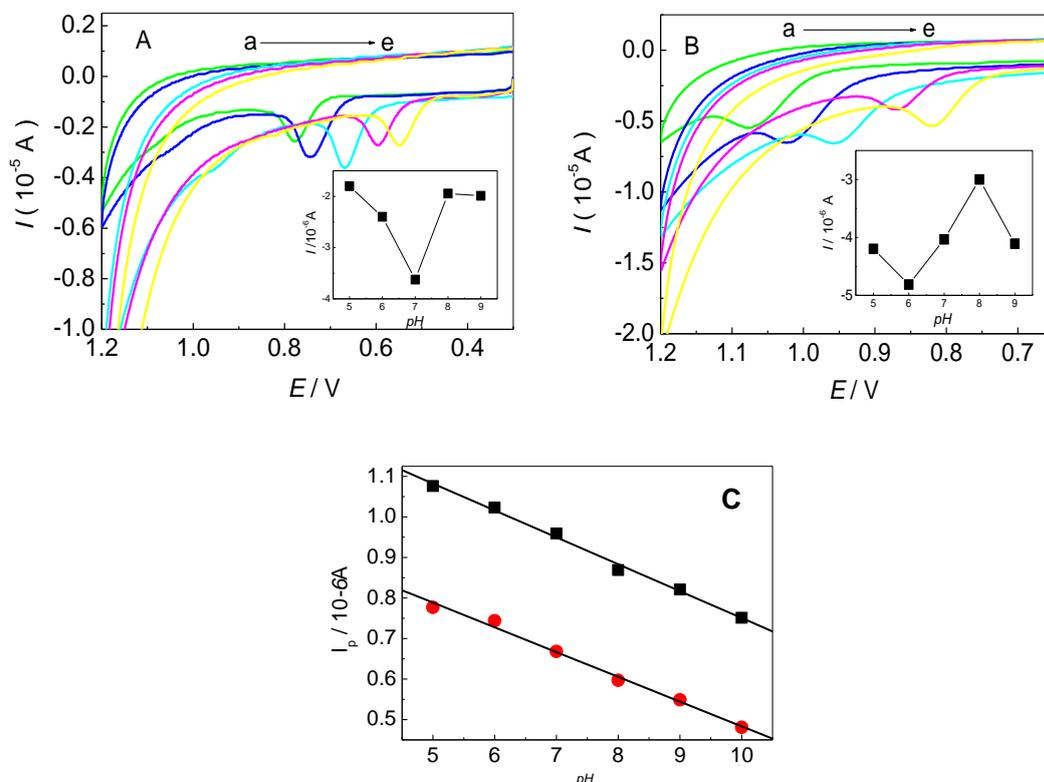
**Figure 5.** CV curves of adenine (A) and guanine (B) with PDA/RGO/GCE in 0.1 M PBS with a scan rate of 100 mV/s at different pH values: a-5.0, b-6.0, c-7.0, d-8.0, and e-9.0. The inset shows the oxidation peak current of adenine and guanine vs. pH. The oxidation peak current of adenine and guanine vs. pH (C).
