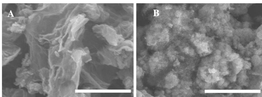
**Figure 2.** SEM images of the different electrodes: A- RGO/GCE and B- PDA/RGO/GCE. Scale bar: 20  $\mu\text{m}$
