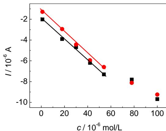
**Figure 8.** Oxidation peak currents of guanine and adenine vs. concentrations.
