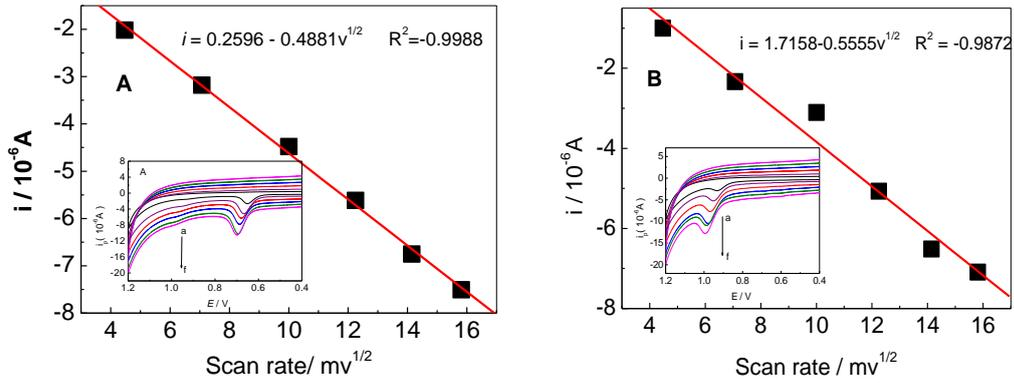
**Figure 6.** Effect of the scan rate on the oxidation peak current of adenine and guanine.
