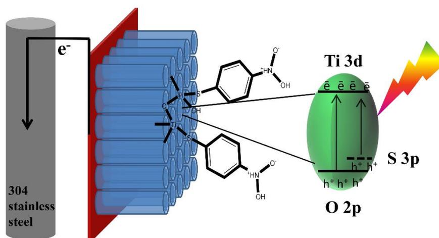
**Figure 9.** A schematic illustration for the fabrication of the 4NBT–TiO<sub>2</sub> NTAs for photocathodic protection of 304 SS.
