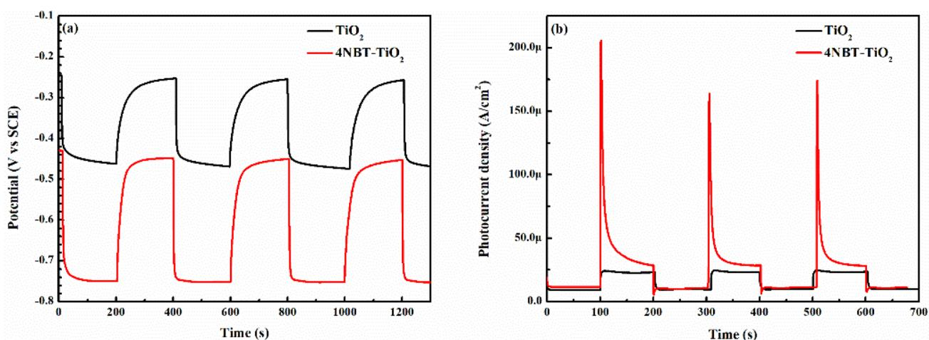
**Figure 8.** (a) The photoinduced variations of the open circuit potentials and (b) variations of the photoinduced current density of the 304 electrode coupled with the synthesized TiO<sub>2</sub> NTAs, 4NBT-TiO<sub>2</sub> NTAs.
