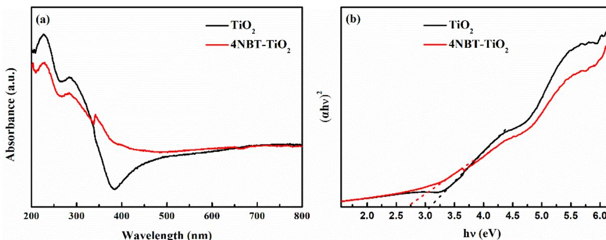
**Figure 5.** (a) UV/Vis diffuse reflectance spectra of the synthesized  $\text{TiO}_2$  NTAs and 4NBT- $\text{TiO}_2$  NTAs and (b) plots of  $(\alpha h\nu)^2$  versus  $h\nu$  for  $\text{TiO}_2$  NTAs and 4NBT- $\text{TiO}_2$  NTAs.
