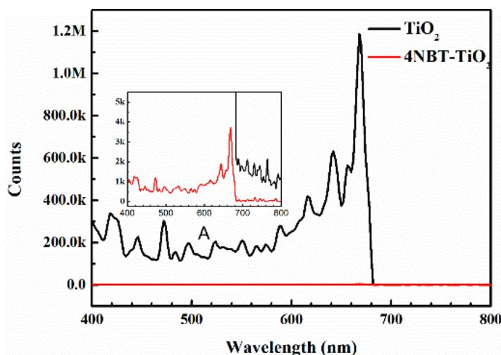
**Figure 6.** Photoluminescence (PL) spectra of the synthesized  $\text{TiO}_2$  NTAs and 4NBT- $\text{TiO}_2$  NTAs with an incident light of 370 nm.
