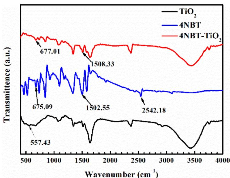
**Figure 4.** IR spectra of 4NBT, the synthesized TiO<sub>2</sub> NTAs, and 4NBT-TiO<sub>2</sub> NTAs.
