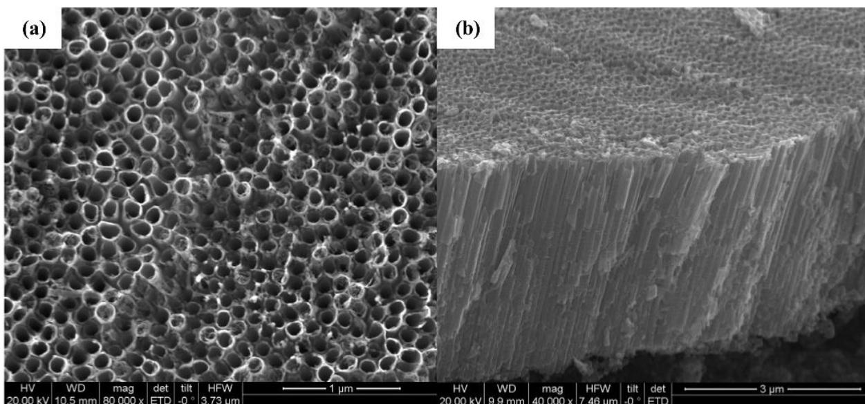
Figure 2. (a) top view SEM image of the as-synthesized TiO<sub>2</sub> NTAs. (b) cross-sectional view SEM image of the as-synthesized TiO<sub>2</sub> NTAs.
