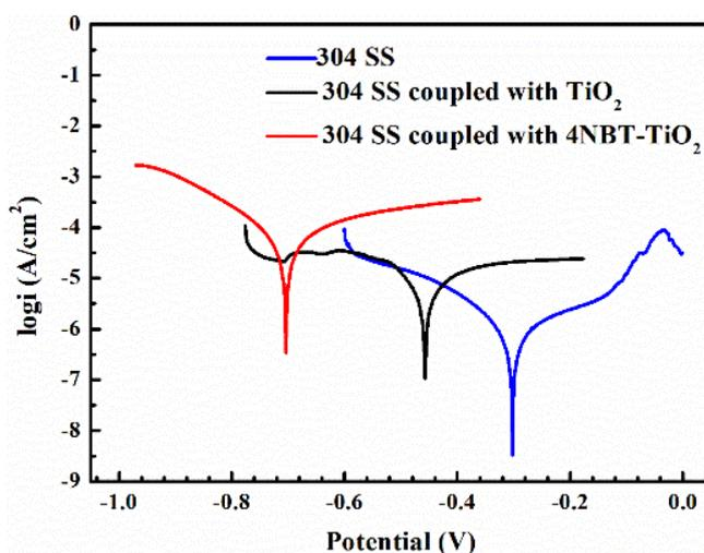
**Figure 7.** Potentiodynamic polarization curves of 304 SS and 304 SS coupled with the synthesized TiO<sub>2</sub> NTAs, 4NBT-TiO<sub>2</sub> NTAs.
