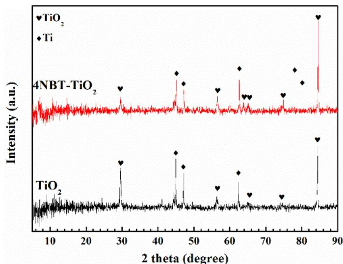
Figure 1. XRD patterns of the pure TiO<sub>2</sub> NTAs and 4NBT–TiO<sub>2</sub> NTAs.
