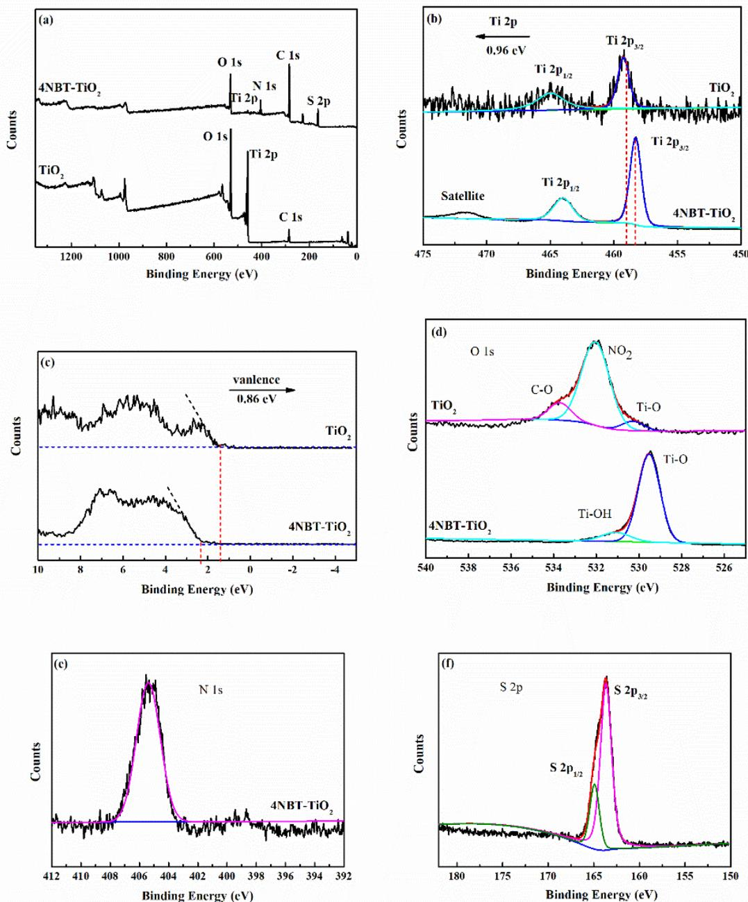
**Figure 3.** XPS survey, Ti 2p, valence, O 1s, N 1s, and S 2p of the surface of the synthesized 4NBT–TiO<sub>2</sub> NTAs.
