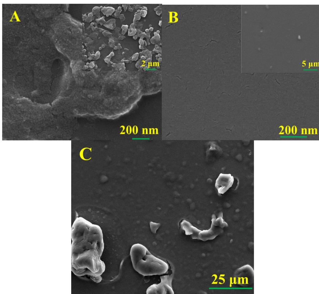
**Figure 1.** SEM images of KVB film (A, magnification, 20,000× and inset magnification, 160,000×), Nf (IP) film (B, magnification, 160,000× and inset magnification, 5000×), KVB-Nf (IP) film (C, magnification, 2000×).
