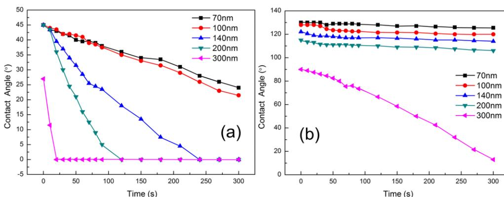
**Figure 4.** Variation of water contact angles on the nanoporous silver surfaces before and after treatment with stearic acid. Dealloying time: 5, 10, 30, 60 and 120 min; electrolyte: 0.1 M H<sub>2</sub>SO<sub>4</sub>; applied voltage: 0.4 V; immersion time in the stearic acid-ethanol solution: 1 min.
