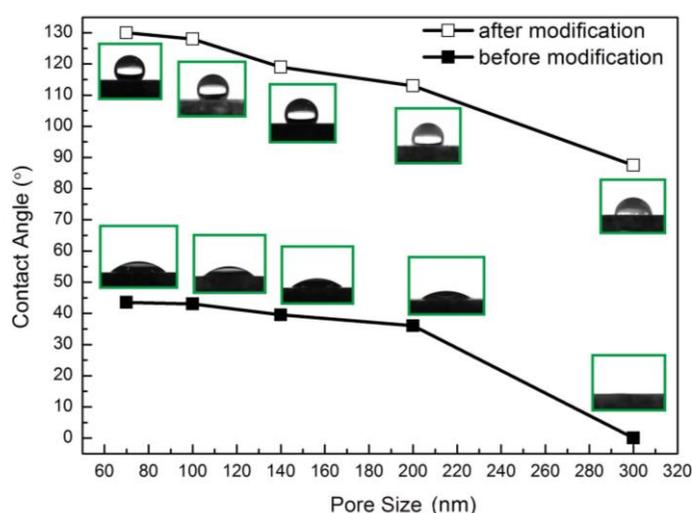
**Figure 2.** Variation of water contact angles on the nanoporous silver surfaces as a function of pore size. Dealloying time: 5, 10, 30, 60 and 120 min; electrolyte: 0.1 M H<sub>2</sub>SO<sub>4</sub>; applied voltage: 0.4 V; immersion time in the stearic acid-ethanol solution: 1 min.
