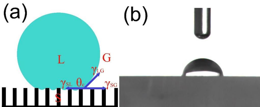
**Figure 3.** (a) Schematic of a water droplet in the Cassie-Baxter state on a rough solid surface, (b) a water droplet with a contact angle of  $79^\circ$  on the smooth silver surface.
