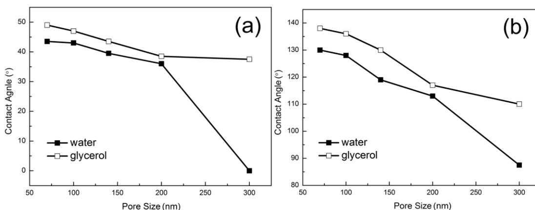
**Figure 6.** Variation of the water and glycerol contact angles on the nanoporous silver surface before and after stearic acid modification as a function of pore size.
