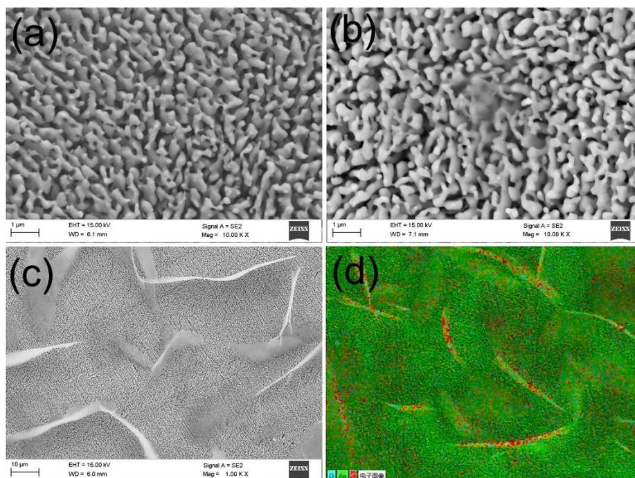
**Figure 1.** Surface morphologies of nanoporous silver immersed in the 0.05 mol/L stearic acid-ethanol solution for (a) 1 min, (b) 5 min, (c) 10 min, and (d) surface element distribution after immersion for 10 min. The nanoporous silver was obtained through dealloying  $\text{Ag}_{25}\text{Zn}_{75}$  for 30 min at 0.4 V in 0.1 M  $\text{H}_2\text{SO}_4$ .
