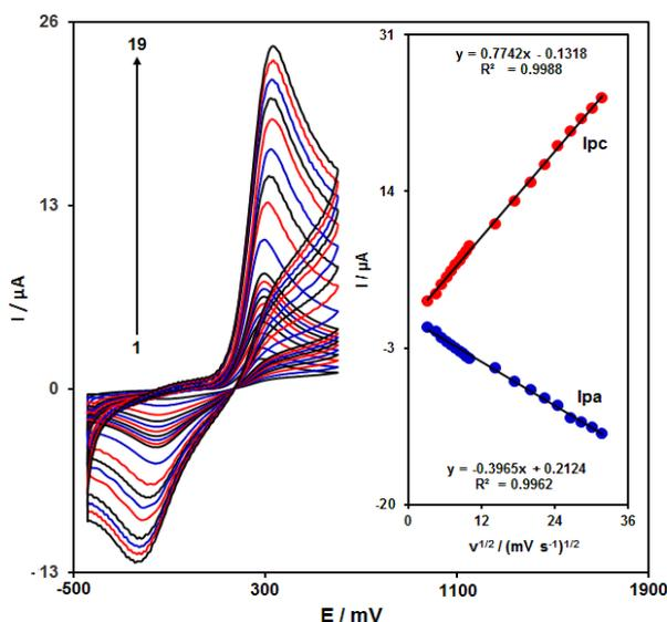
**Figure 2.** CVs of MTD/SPE in 0.1 M PBS at pH of 7.0 consisting of 150.0  $\mu\text{M}$  acetaminophen at distinct scan rates; 1-9 corresponded to 10, 20, 30, 40, 50, 60, 70, 80, 90, 100, 200, 300, 400, 500, 600, 700, 800, 900 and 1000  $\text{mV s}^{-1}$ . Inset; variations in the anodic peak currents vs.  $v^{1/2}$ .
