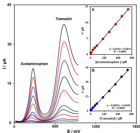
**Figure 6.** The DPV of the MTD/SPE in 0.1 M PBS at pH of 7.0 with various concentrations of acetaminophen + tramadol. Notably, 1–7 corresponded to 5.0+5.0, 15.0+15.0, 40.0+40.0, 70.0+70.0, 100.0+100.0, 200.0+200.0, 300.0+300.0, 400.0+400.0, 500.0+500.0 and 600.0+600.0  $\mu\text{M}$  of acetaminophen and tramadol. Inset A. The  $I_p$  plot vs. acetaminophen concentration. B. The  $I_p$  plot vs. tramadol concentration.
