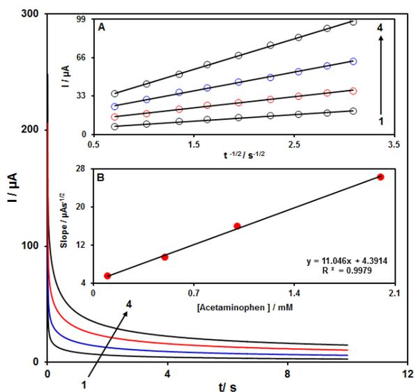
**Figure 4.** The chrono-amperograms obtained at MTD/SPE in 0.1 M PBS at pH of 7.0 for different concentrations of acetaminophen. It is notable that 1–4 correspond to 0.1, 0.4, 0.8, 1.3 and 2.0 mM of acetaminophen. Inset A. the  $I$  plot versus  $t^{-1/2}$  observed by chrono-amperograms 1 to 4. B. Slope plot of the straight line vs. concentration of acetaminophen.
