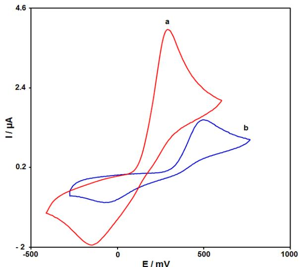
**Figure 1.** The CVs of a) MTD/SPE, (b) unmodified SPE in 0.1 M PBS at pH of 7.0 in the presence of 100.0  $\mu\text{M}$  acetaminophen at  $50 \text{ mVs}^{-1}$  scan rate.
