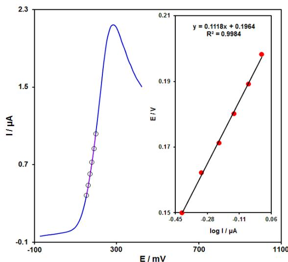
**Figure 3.** The linear sweep voltammograms at  $10 \text{ mV s}^{-1}$  of the electrodes in 0.1 M PBS at pH equal to 7.0) with  $150.0 \text{ } \mu\text{M}$  acetaminophen. These points stand for the output utilized in Tafel plot. As seen, inset represents Tafel plot derived from the linear sweep voltammogram.
