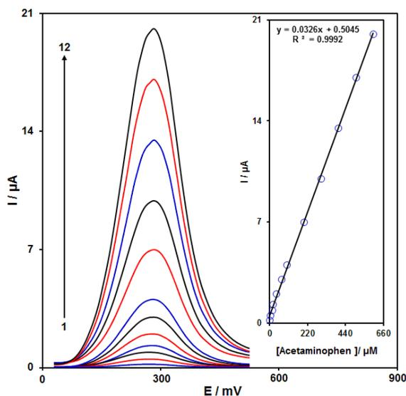
**Figure 5.** DPVs of MTD/SPE in 0.1 M PBS (pH 7.0) containing different concentrations of acetaminophen. Numbers 1–12 correspond to 0.04, 5.0, 15.0, 20.0, 40.0, 70.0, 100.0, 200.0, 300.0, 400.0, 500.0 and 600.0  $\mu\text{M}$  of acetaminophen. The inset shows the plot of the peak current as a function of the acetaminophen concentration in the range of 0.040-600.0  $\mu\text{M}$ .
