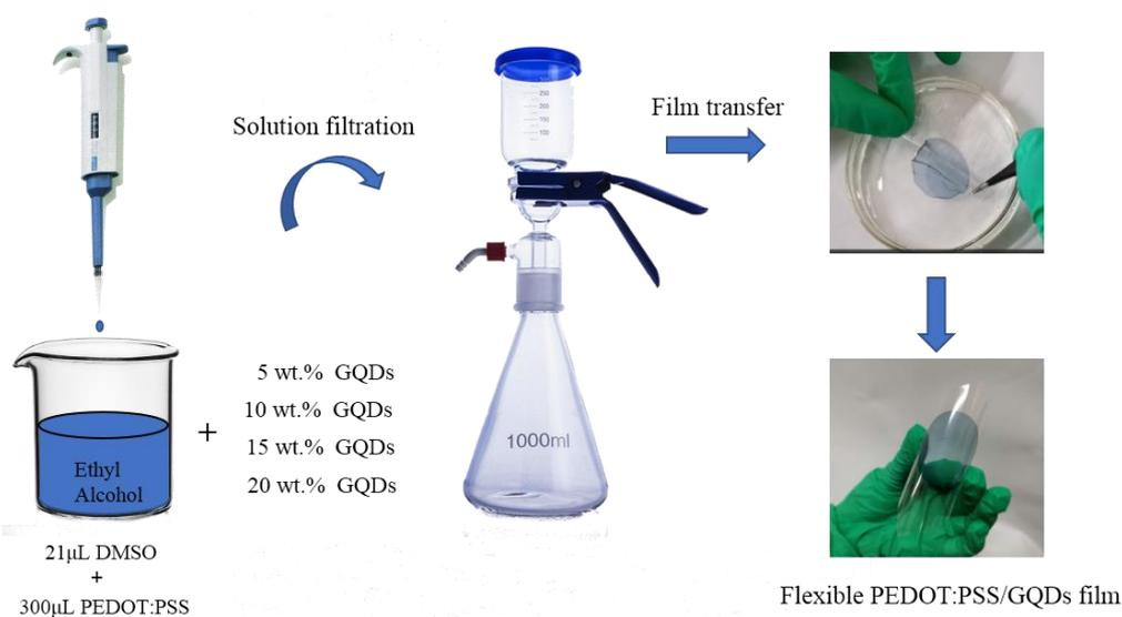
**Figure 1.** Schematics of the process for fabricating the PEDOT:PSS/GQDs film.
