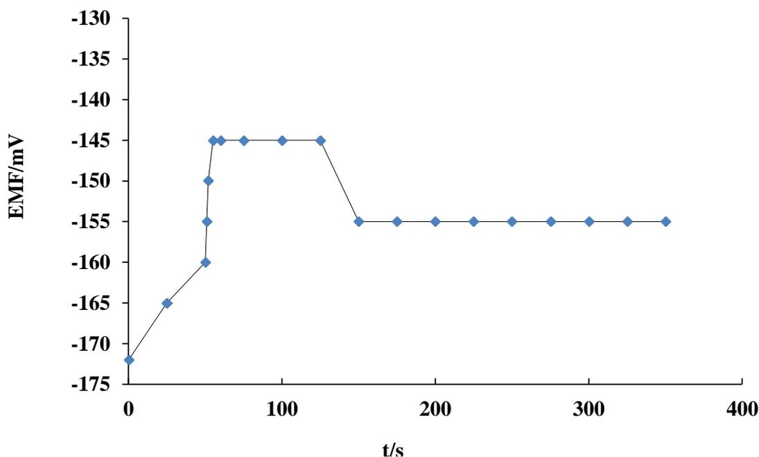
**Figure 2.** The response time of the sensor in magnesium ions concentration [ 10<sup>-6</sup> - 10<sup>-1</sup> M ].
