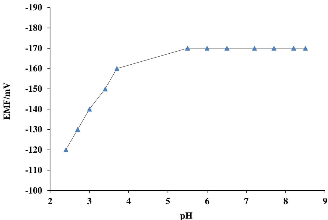
**Figure 3.** pH dependence of the sensor response in magnesium ions concentration [  $10^{-6}$  -  $10^{-1}$  M ].
