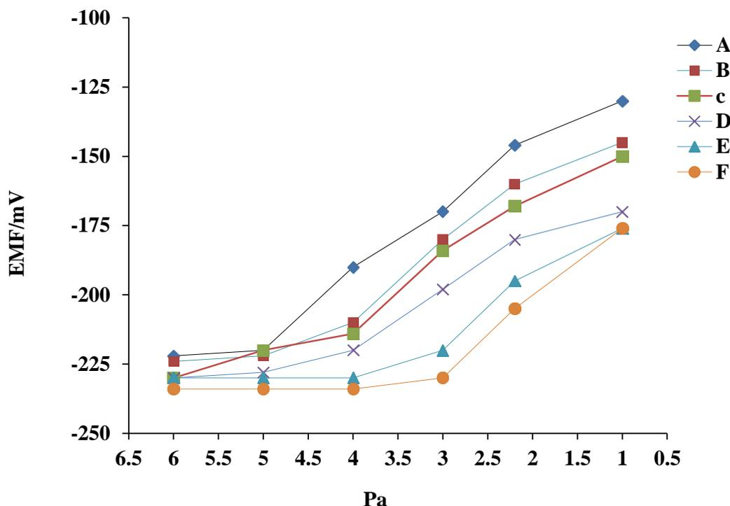
**Figure 1.** Calibration curves of magnesium sensor, ( A ) Mg, (B) Cu, (C) Cd, (D) Ni, (E) Co and (F) Ca cations estimated in magnesium and its interfering ions of  $10^{-6}$ - $10^{-1}$  molar solutions
