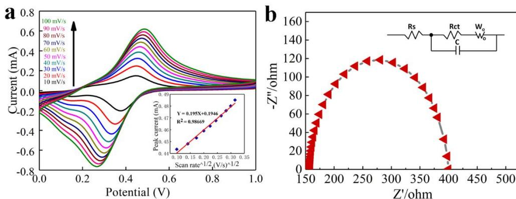
**Figure 3.** (a) CV curves of PSTF in a potential range of 0~1.0 V at various scan rates from 10 to 100 mV/s. The inset shows the relationship curve between the peak current and the square root of the scan rate. (b) EIS of PSTF in 0.1 M HCl electrolyte solution.
