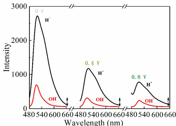
**Figure 6.** Fluorescence switching of PSTF/ITO electrode when immersed into the acid solution and alkaline solution alternately. The redox state of tetraaniline units in PSTF structure was fixed by the potentiostatic method at voltages of 0 V, 0.4 V, and 0.8 V.
