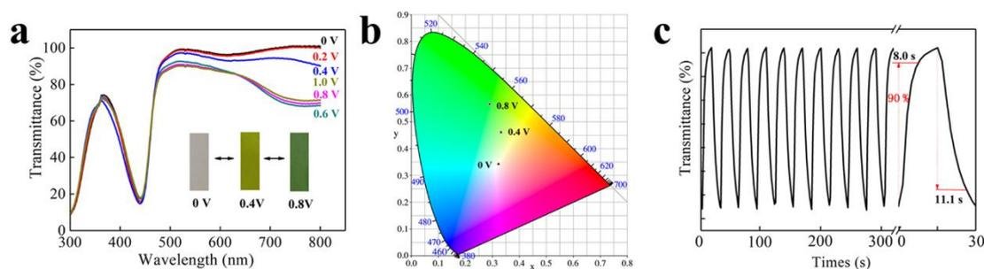
**Figure 4.** (a) Transmittance spectra of PSTF film under various voltages with a residence time of 200 s. Inset reveals the photographs under various applied voltages. (b) The CIE 1931(x, y) chromaticity diagram of the PSTF films at different potentials. (c) Optical change of PSTF film collected at 750 nm under voltages of 0 V and 0.6 V, and its switching times during the color switching.
