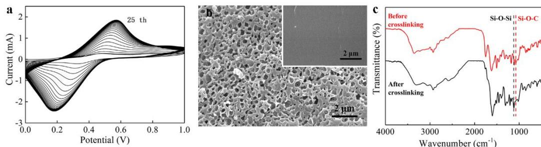
Figure 2. (a) CV curves of siloxane precursors mixture in the potential range of 0~1.0 V at 100 mV/s. (b) SEM morphology of PSTF after hydrolysis, and the inset shows the SEM morphology of siloxane precursors mixture before hydrolysis. (c) FTIR spectra of siloxane precursors mixture and PSTF.
