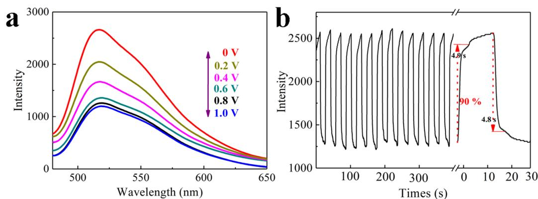
**Figure 5.** (a) Fluorescence spectra of PSTF film under various voltages (0.0-1.0 V). (b) Fluorescence change at 517 nm of PSTF coating under repeated applied voltages of 0 V and 1.0 V. The excitation wavelength is fixed at 425 nm.
