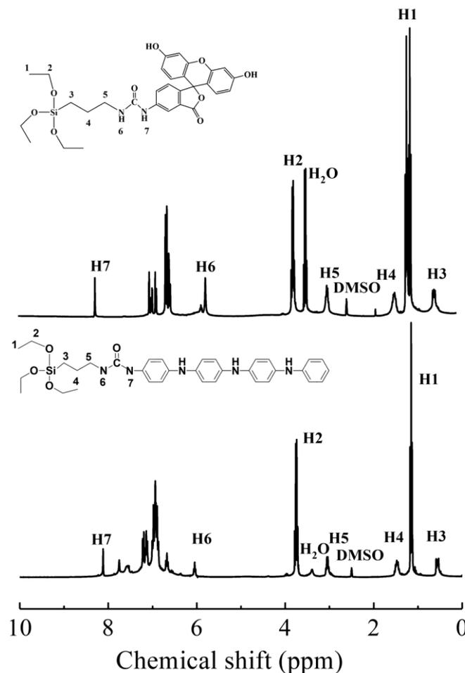
Figure 1. <sup>1</sup>H NMR spectra of Si-TA and Si-F.
