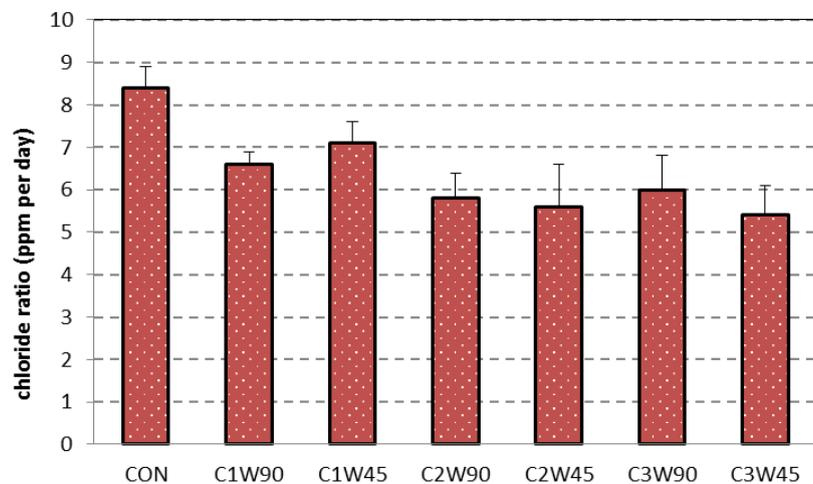
**Figure 5.** Chloride ratio (ppm per day) in various samples with CFP in different wrap fiber orientation and different number of CFP layers at room temperature
