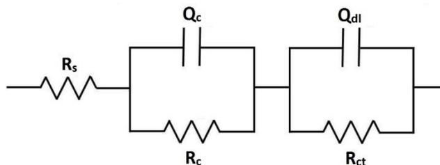
**Figure 7.** Equivalent circuit model used
