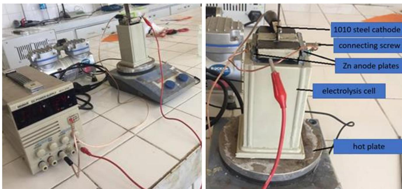
**Figure 1.** The experimental setup in which Zn coating was performed
