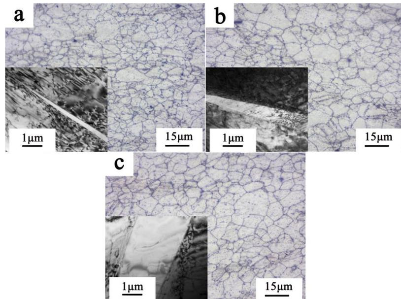
**Figure 2.** Microstructure comparison (metallography and TEM); (a) 250 °C rolled sheet; (b) 300 °C rolled sheet; (c) 350 °C rolled sheet
