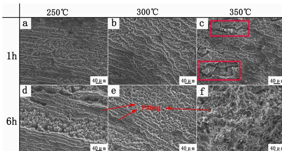
**Figure 6.** Corrosion morphologies of magnesium alloy sheet rolled at 250 °C, 300 °C and 350 °C; (a, b, c) Soaking for 1 h; (d, e, f) Soaking for 6 h (3.5 wt% NaCl solution)
