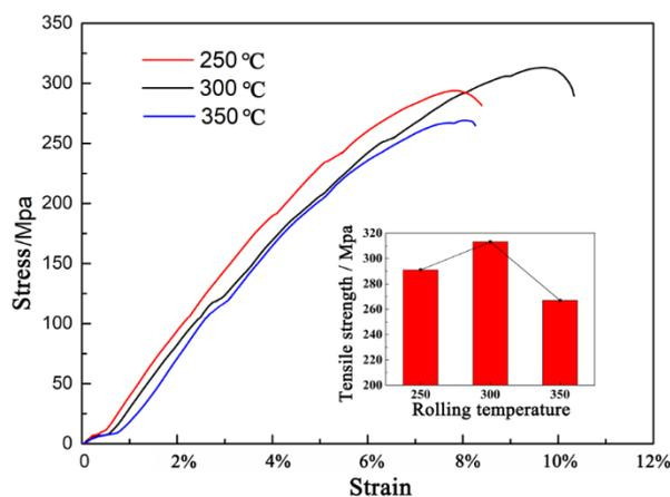
**Figure 7.** Stress-strain curves and tensile strength of magnesium alloy sheet rolled at 250 °C, 300 °C and 350 °C (Strain rate  $1.0 \times 10^{-4} \text{ s}^{-1}$ )
