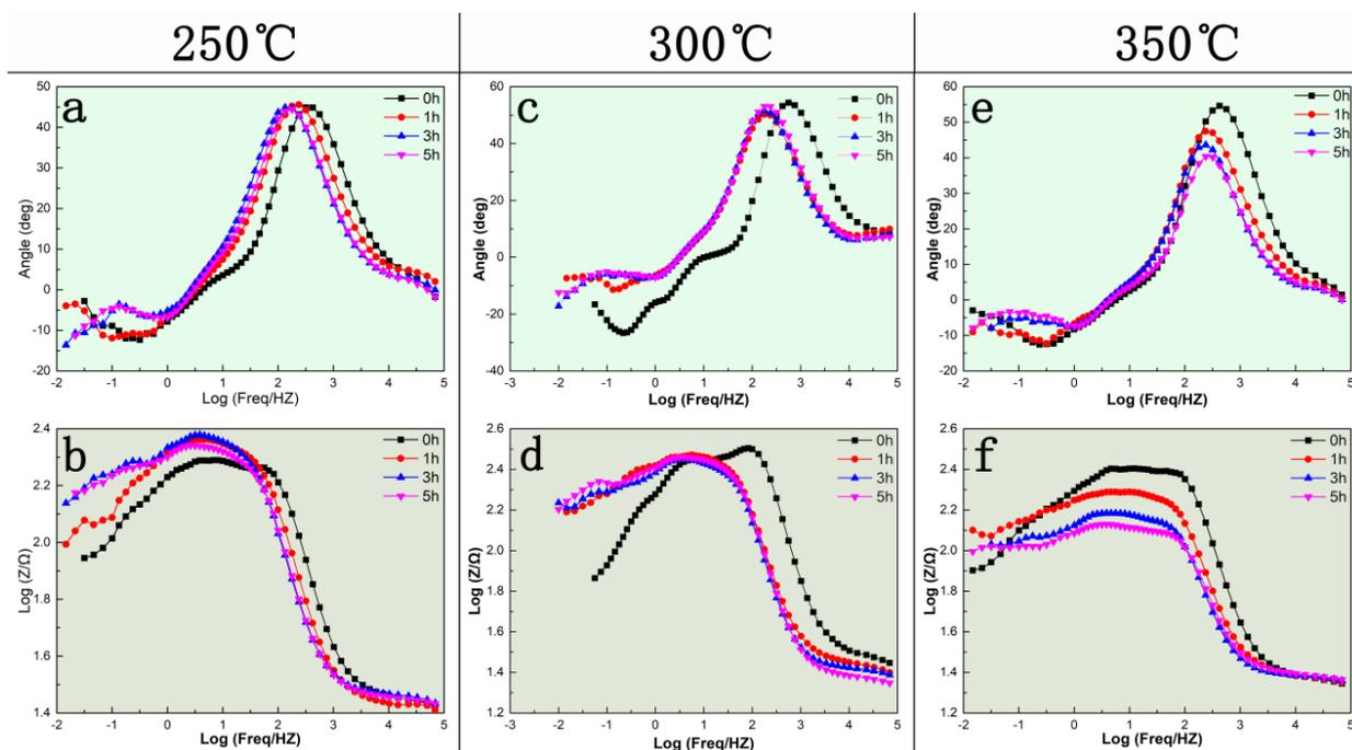
**Figure 5.** Bode plots; (a-b) 250 °C rolled sheet; (c-d) 300 °C rolled sheet; (e-f) 350 °C rolled sheet (3.5 wt% NaCl solution, 1 mHz~100 KHz frequency range, 5-10 mV sinusoidal wave)
