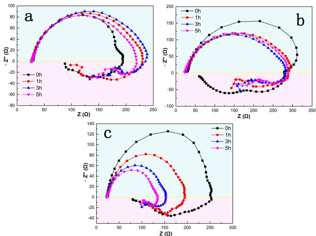
**Figure 5.** Nyquist plots; (a) 250 °C rolled sheet; (b) 300 °C rolled sheet; (c) 350 °C rolled sheet (3.5 wt% NaCl solution, 1 mHz~100 KHz frequency range, 5-10 mV sinusoidal wave)
