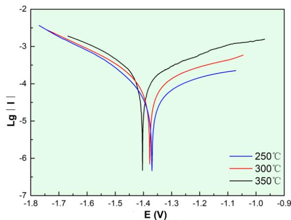
**Figure 3.** Polarization curves of magnesium alloy rolled at 250 °C, 300 °C and 350 °C (3.5 wt% NaCl solution, 0.05 mV/s scanning rate, 0.001 s sampling interval)
