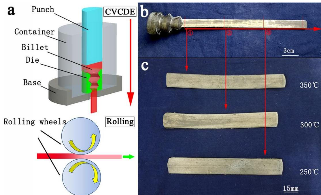
**Figure 1.** Magnesium alloy sheet and its forming process; (a) CVCDE and rolling; (b) CVCDEed sheet (350 °C extrusion temperature); (c) Rolled sheets at 250 °C, 300 °C and 350 °C
