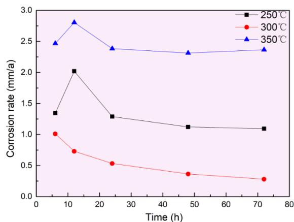
**Figure 4.** Corrosion rate curves of magnesium alloy rolled at 250 °C, 300 °C and 350 °C (3.5 wt% NaCl solution, soaking time: 6 h, 12 h, 24 h, 48 h and 72 h)
