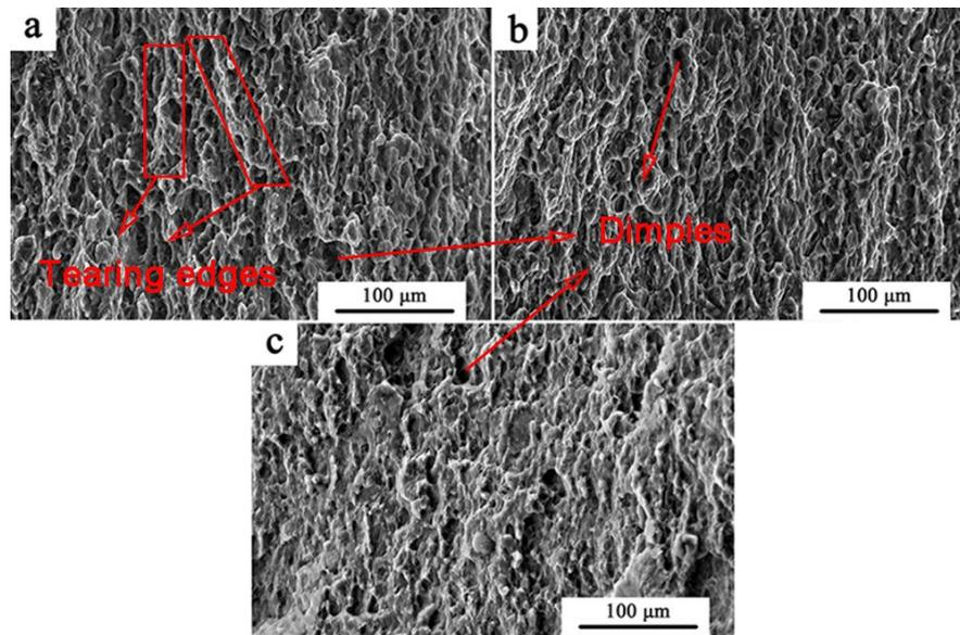
**Figure 8.** Fracture morphologies of magnesium alloy sheet rolled at 250 °C, 300 °C and 350 °C; (a) 250 °C rolled sheet; (b) 300 °C rolled sheet; (c) 350 °C rolled sheet
