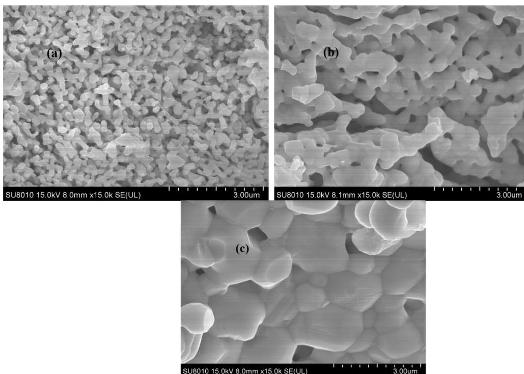
**Figure 3.** The SEM pictures of  $\text{La}_2\text{CuO}_4$  sintered at different temperatures (a) 800 °C, (b) 900 °C, (c) 1100 °C.
