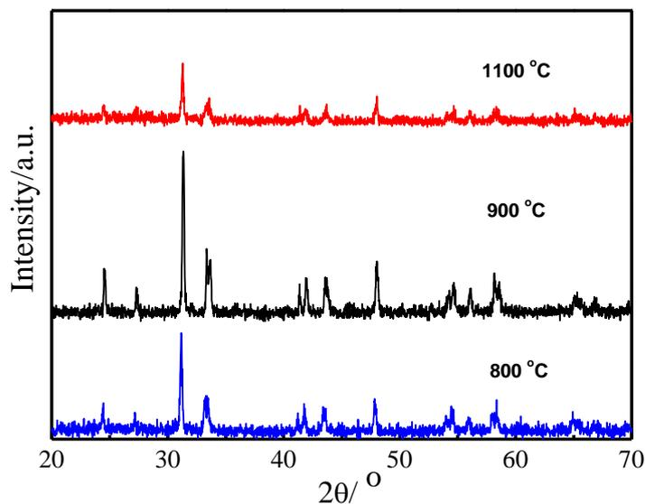
**Figure 2.** The crystal structure of  $\text{La}_2\text{CuO}_4$  sintered at different temperatures.
