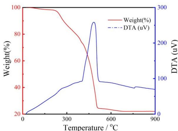
**Figure 1.** TG-DTA curve of the xerogel to 900 °C.
