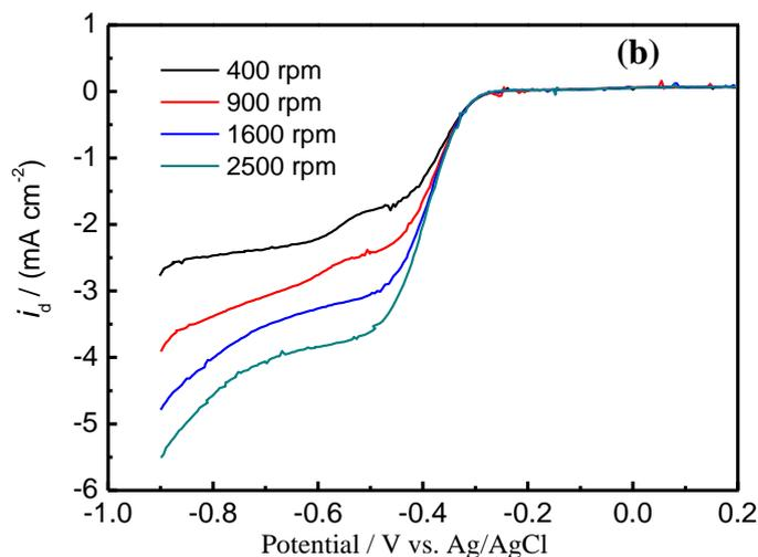
**Figure 6.** The disk ( $i_d$ ) current densities ~ potential curves in 0.1 M KOH solution at four different rotation speeds (400, 900, 1600 and 2500 rpm) of  $\text{La}_2\text{CuO}_4@Au$  (a) and  $\text{La}_2\text{CuO}_4$  (b) during oxygen reduction reaction (ORR).
