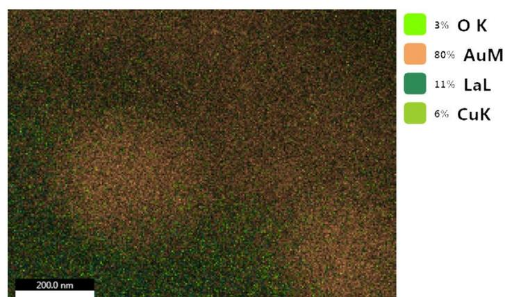
**Figure 4.** The EDS Mapping analysis of  $\text{La}_2\text{CuO}_4@Au$ .
