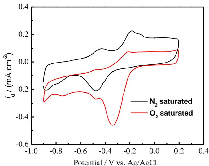
**Figure 5.** The cyclic voltammetric (CV) curves of the bifunctional oxygen electrode in 0.1 M KOH electrolyte. The scanning range of potential is - 1.0 V ~ 0.4V under the N<sub>2</sub> or O<sub>2</sub> saturated conditions.
