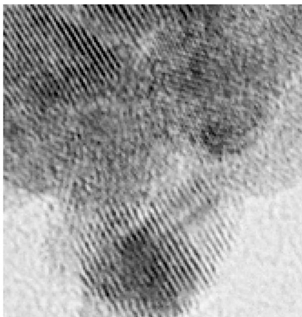
**Figure 5.** TEM of spherical  $\text{CeO}_2$  nanospheres doped with 5wt% Pt. Reprinted with permission from reference [58]. Copyright 2009 American Chemical Society.
