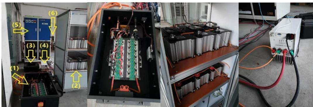
**Figure 6.** The 72V hybrid system test bench, which consists of a battery pack as main source, a supercapacitor pack as aided source, a RapidECU for algorithm implement, a DC/DC converter for power flow regulation, a load simulator for cycle simulation, and a personal computer.
