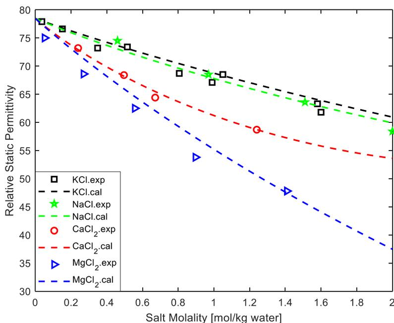
**Figure 1.** Relative static permittivity of aqueous electrolyte solutions at 298.15 K.
