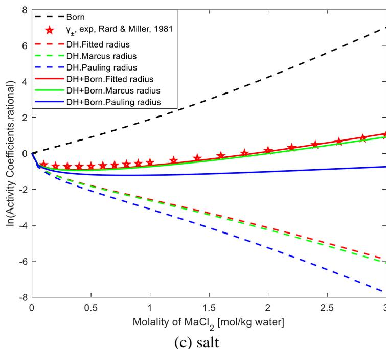
**Figure 5.** Contributions of the activity coefficients for ions and salt in aqueous  $\text{MgCl}_2$  solution.
