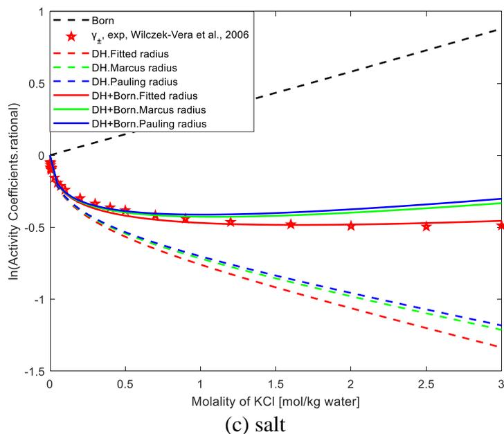
**Figure 3.** Contributions of the activity coefficients for ions and salt in aqueous KCl solution.
