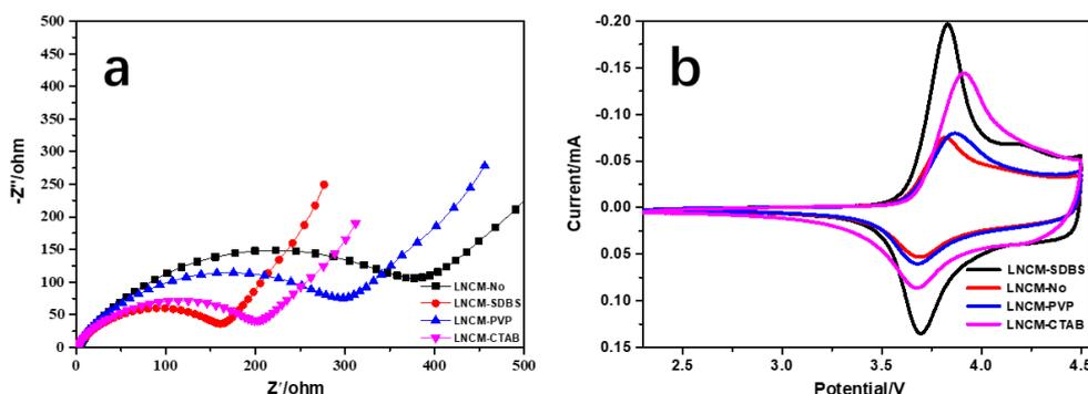
Figure 6. The EIS and CV curves of cathode materials with different surfactants addition
