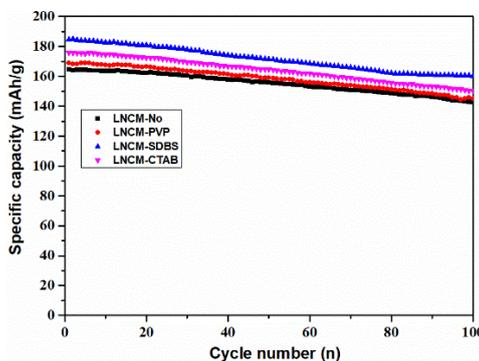
**Figure 3.** Cycle performance of cathode materials with different surfactants
