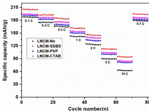
**Figure 4.** Rate performances of cathode materials with different surfactants
