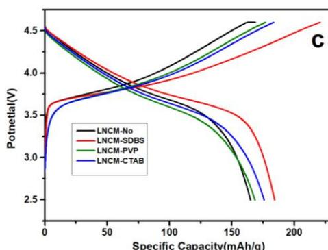
**Figure 5** Initial charge and discharge curves of cathode materials with different surfactants at 0.5 C
