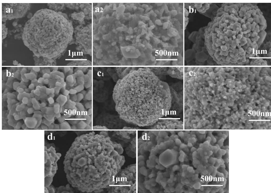
**Figure 2.** SEM images of synthetic NCM materials. (a<sub>1</sub>, a<sub>2</sub>) without surfactant, (b<sub>1</sub>, b<sub>2</sub>) with SDBS, (c<sub>1</sub>, c<sub>2</sub>) with PVP, (d<sub>1</sub>, d<sub>2</sub>) with CTAB
