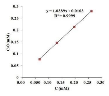
**Figure 3.** Langmuir adsorption isotherm of pantoprazole calculated by potentiodynamic polarization data for carbon steel in 3.5% NaCl solution saturated with CO<sub>2</sub>.
