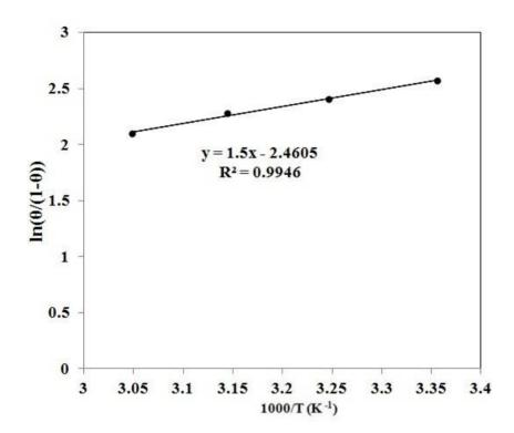
**Figure 9.** Plot of  $\ln (\theta/1-\theta)$  vs. 1/T for carbon steel in CO<sub>2</sub> saturated brine solution containing 100 ppm pantoprazole.
