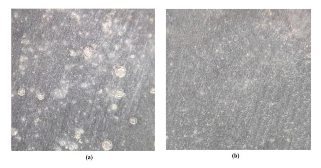
**Figure 10.** The optical microscopy images of sand-covered carbon steel electrode after 1 h from immersion in CO<sub>2</sub> saturated brine solution in (a) the absence and (b) presence of 100 ppm pantoprazole drug.
