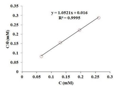
**Figure 6.** Langmuir adsorption isotherm of pantoprazole calculated on the basis of EIS data for carbon steel in 3.5% NaCl solution saturated with CO<sub>2</sub>.
