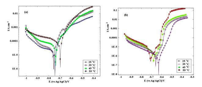
**Figure 7.** Effect of temperature on the polarization curves of carbon steel in CO<sub>2</sub> saturated brine solution (a) without pantoprazole drug and (b) in the presence of 100 ppm pantoprazole drug.
