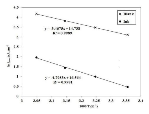
**Figure 8.** Arrhenius plots for carbon steel in CO<sub>2</sub> saturated brine solution in the absence (Blank) and presence of 100 ppm pantoprazole (Inh).
