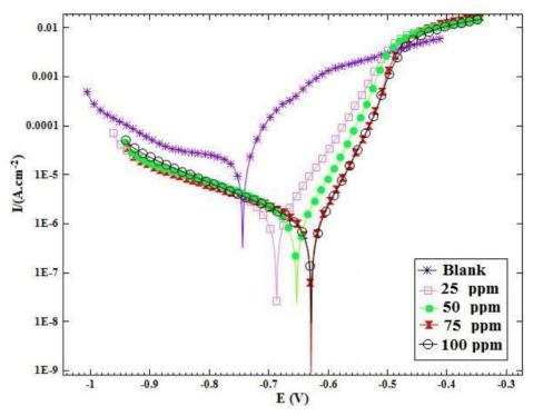
**Figure 2.** Polarization curves of carbon steel in CO<sub>2</sub> saturated brine solution containing different concentrations of pantoprazole at 25°C.
