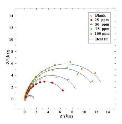
**Figure 4.** Nyquist plots for carbon steel in 3.5% NaCl solution saturated with CO<sub>2</sub> containing different concentrations of pantoprazole at 25°C.
