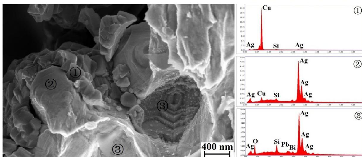
**Figure 4.** EDS of the grid electrode on the recycled c-Si solar cell after Ag/Cu plating repair.
