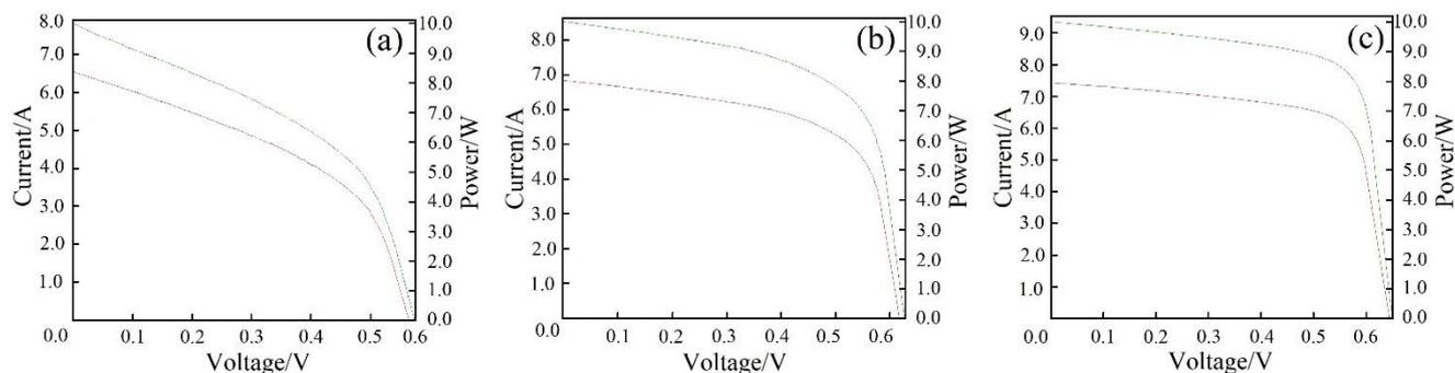
**Figure 5.** I-V curves of the recycled c-Si solar cells; (a) before repair; (b) after Ag light-induced plating; (c) after Cu plating.
