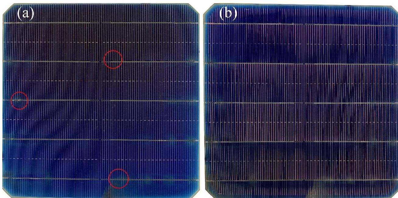
**Figure 7.** The pictures of c-Si solar cells. (a) Before Ag/Cu plating repair; (b) After Ag/Cu plating repair.
