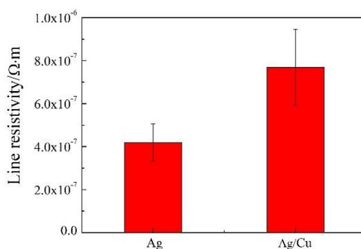
**Figure 6.** The line resistivity of the repaired electrodes with Ag plating and Ag/Cu plating.
