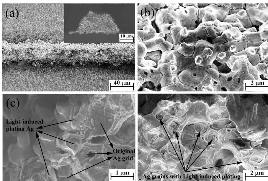
**Figure 2.** SEM images of Ag electrodes after Ag light-induced plating, (a) the surface of the Ag grid and the inset is the cross-section of the Ag grid; (b) magnified surface of the Ag grid; (c) and (d) magnified cross-section of the Ag grid.
