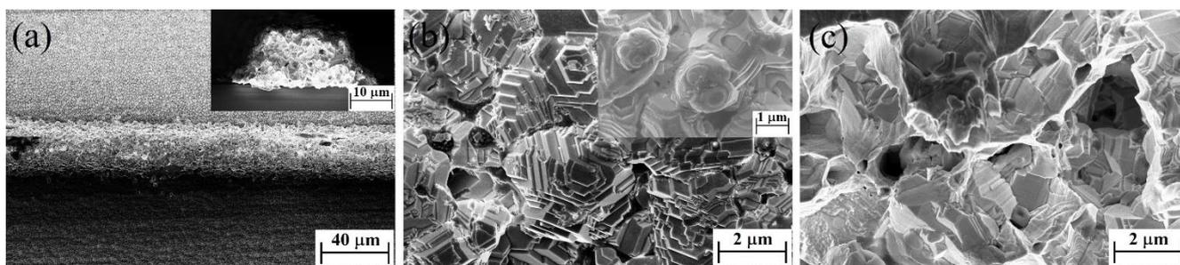
**Figure 1.** SEM images of Ag electrodes before repair, (a) the surface of the Ag grid and the inset is the cross-section of the Ag grid; (b) the magnified surface of the Ag grid and the inset is the surface of the sintered Ag particles; (c) the magnified cross-sectional image of the Ag grid.
