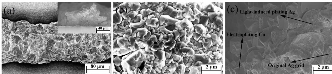
**Figure 3.** SEM images of Ag electrodes after Cu electroplating, (a) the surface of the Ag grids and the inset is the cross-section of the Ag grids; (b) magnified surface of the Ag grids; (c) magnified cross-section of the Ag grids.
