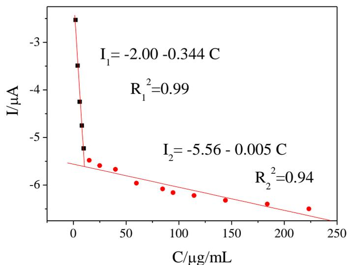
**Figure 4.** Corresponding linear calibration curve of peak current vs. benzylpenicillin concentration.
