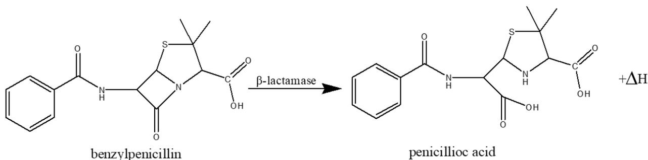
**Figure 5.** The reaction of the hydrolytic degradation of the four-membered  $\beta$ -lactam ring.
