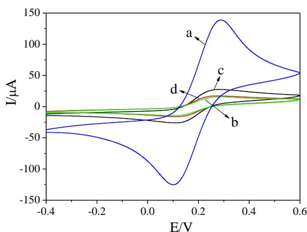
**Figure 2.** CVs of the bare GE, BLM/GE, C<sub>60</sub>-s-BLM, β-lactamase/C<sub>60</sub>-s-BLM/GE in 1 mM [Fe(CN)<sub>6</sub>]<sup>3-/4-</sup> (1:1) solution with a scan rate of 100 mV s<sup>-1</sup>.
