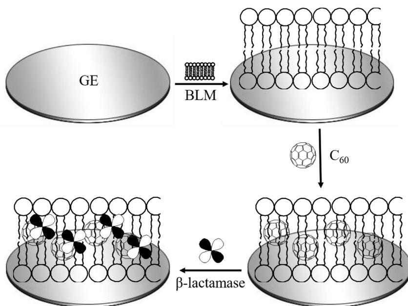
**Scheme 1.** The schematic illustration of the stepwise procedure of the biosensor fabrication.
