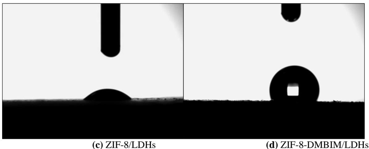
**Figure 6.** Water drop morphology on AZ61 substrate, ZnAl-NO<sub>3</sub> LDHs, ZIF-8/LDHs and ZIF-8-DMBIM/LDHs film during the static contact angle measurement.
