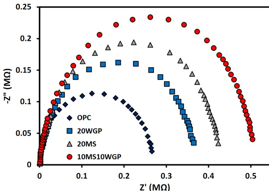
**Figure 4.** EIS diagram of steel rebar embedded in concrete with partial replacement of OPC by WGP and MS after four-week exposure time in 3.5 wt% NaCl solution
