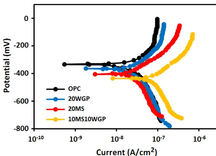
**Figure 6.** Polarization of steel rebar in different concrete samples exposed to 3.5 wt% NaCl solution after four weeks exposure time
