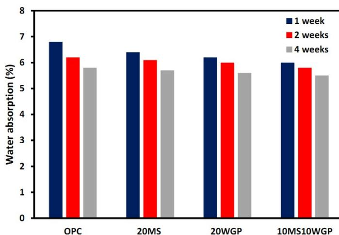
**Figure 3.** Water absorption of partial replacement of OPC with WGP and MS after 1, 2 and 4 weeks exposed to a marine environment.
