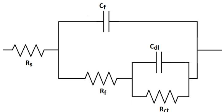
**Figure 5.** Fitted circuit model with the experimental data
