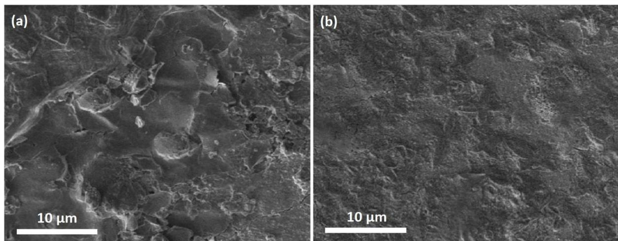
**Figure 6.** FESEM images of carbon steel rebar embedded in (a) OPC and (b) mixtures containing 10 % MS and 10 % WGP after 4-weeks immersion time into 3.5 wt% NaCl solution
