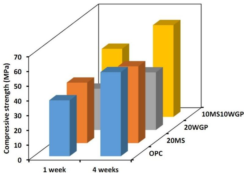
**Figure 2.** Compressive strength of partial replacement of OPC with WGP and MS.
