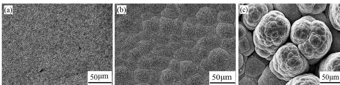
**Figure 13.** Morphological changes in the deposit surface under the influence of the current density: (a)  $150 \text{ A/dm}^2$ ; (b)  $300 \text{ A/dm}^2$ ; (c)  $450 \text{ A/dm}^2$
