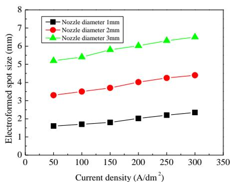
**Figure 10.** Effect of the current density on the electroformed spot size
