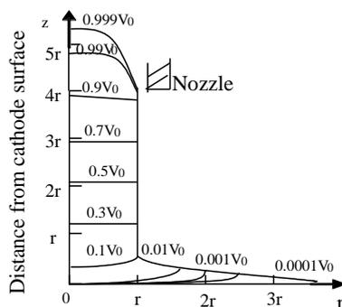
**Figure 4.** Calculated potential distribution in the impinging jet-affected zone
