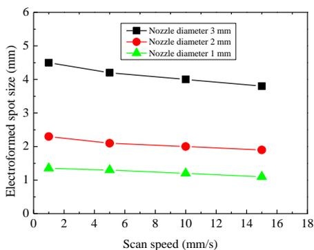
**Figure 11.** Effect of the nozzle scan speed on the electroformed spot size
