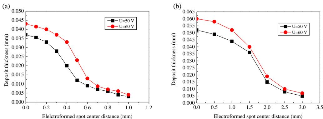
**Figure 6.** Thickness distribution of the deposit thickness with different nozzle diameters: (a) 1 mm; (b) 3 mm
