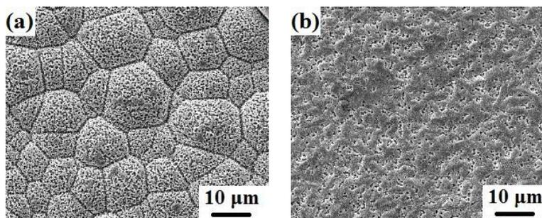
**Figure 7.** SEM appearance of the surface at different positions of casting spots with (a) the electroforming spot centre and (b) the electroforming spot edge
