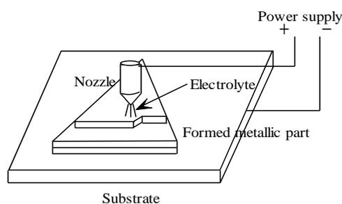
**Figure 2.** Schematic diagram of electrolyte jet machining based on rapid prototyping
