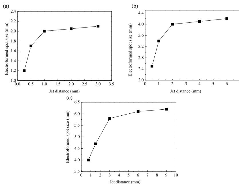
**Figure 8.** Effect of the spray distance on the size of the electroformed spot with different nozzle diameters: (a) 1 mm; (b) 2 mm; (c) 3 mm
