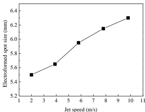
**Figure 12.** Influence of the jet speed on the electroformed spot size
