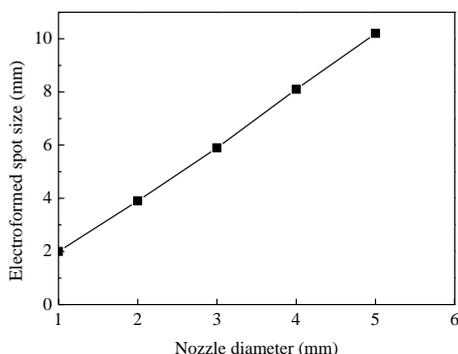
**Figure 5.** Effect of the nozzle diameter on the electroformed spot size
