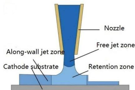
**Figure 1.** Schematic diagram for a typical electrolyte jet machining process
