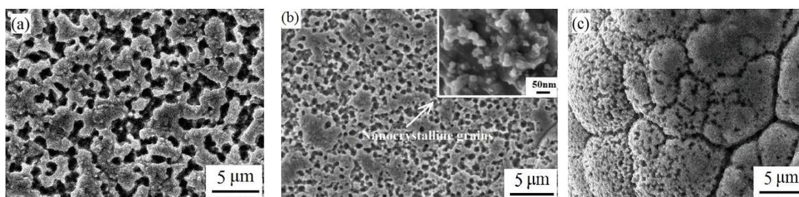
**Figure 14.** Microstructural changes in the deposit layer under the influence of the current density: (a)  $150 \text{ A/dm}^2$ ; (b)  $300 \text{ A/dm}^2$ ; (c)  $450 \text{ A/dm}^2$
