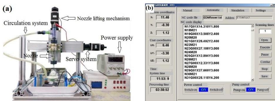
Figure 3. Electrolyte jet machining rapid prototyping system: (a) experimental setup and (b) control software interface
