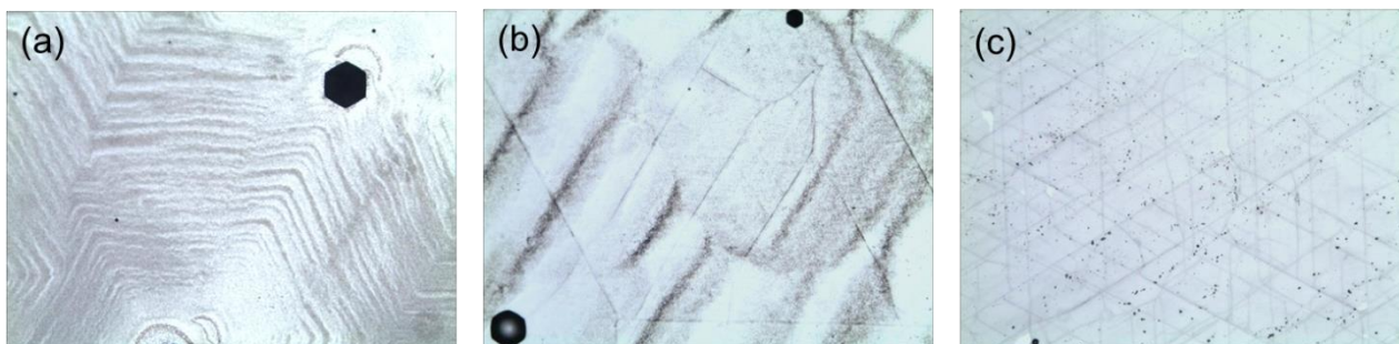
Figure 1. Microscope images of GaN grown at (a) V/III=10, (b) V/III=20, and (c) V/III=50.
