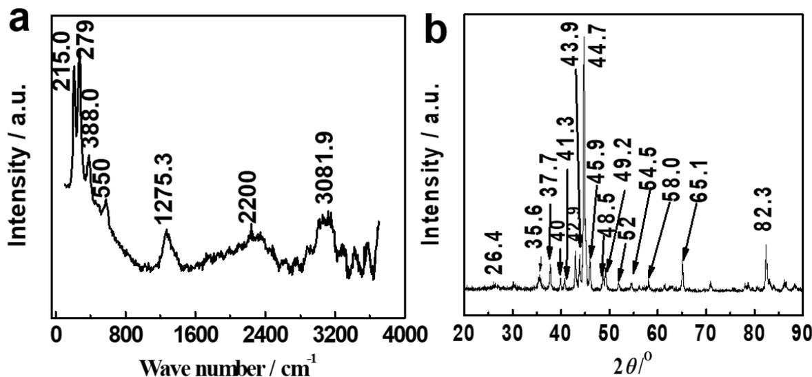
**Figure 7.** (a) Raman spectra, (b) XRD pattern of Fe<sub>3</sub>-600.
