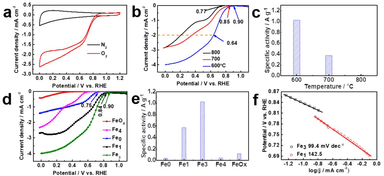
**Figure 3.** (a) CV curves for Fe<sub>3</sub>-600 in N<sub>2</sub>- and O<sub>2</sub>-saturated electrolyte, (b) LSV curves for ORR of Fe<sub>3</sub>-600, 700 and 800, (c) specific activity for ORR with various temperature, the current at 0.80 V<sub>RHE</sub>, (d) LSV curves for ORR of sample with various Fe content, (e) specific activity for ORR with various Fe content at 0.80 V<sub>RHE</sub>, (f) Tafel plots for Fe<sub>3</sub> and Fe<sub>1</sub>.
