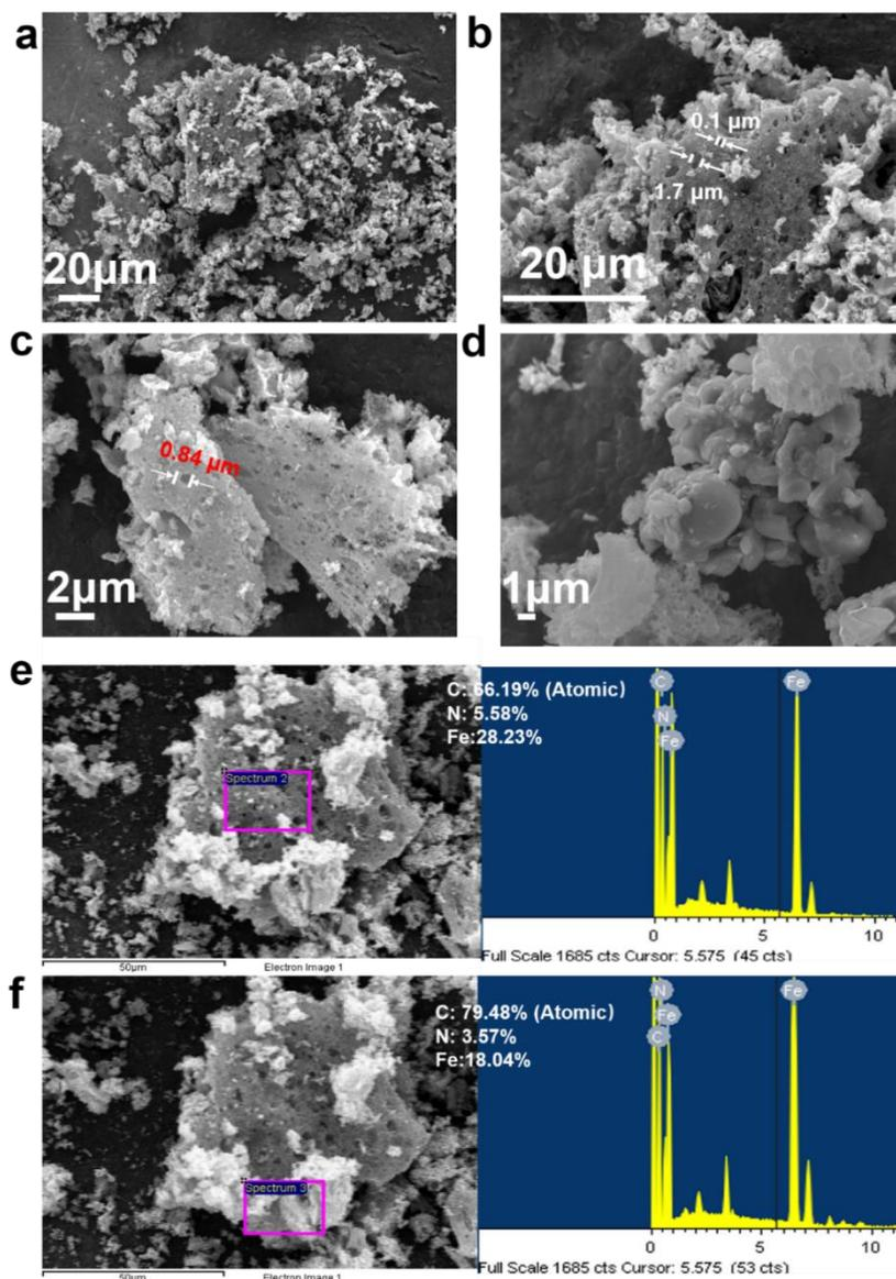
**Figure 5.** SEM images of Fe<sub>3</sub>-600, (a) preliminary image of the sample, (b) image at higher magnification, (c) image of the white solids, (d) image of Fe<sub>3</sub>-800, (e) EDX spectra of Fe<sub>3</sub>-600 of grey zone and (f) white zone.
