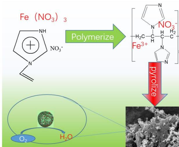
**Figure 2.** Schematic illustration of the catalyst preparation process.
