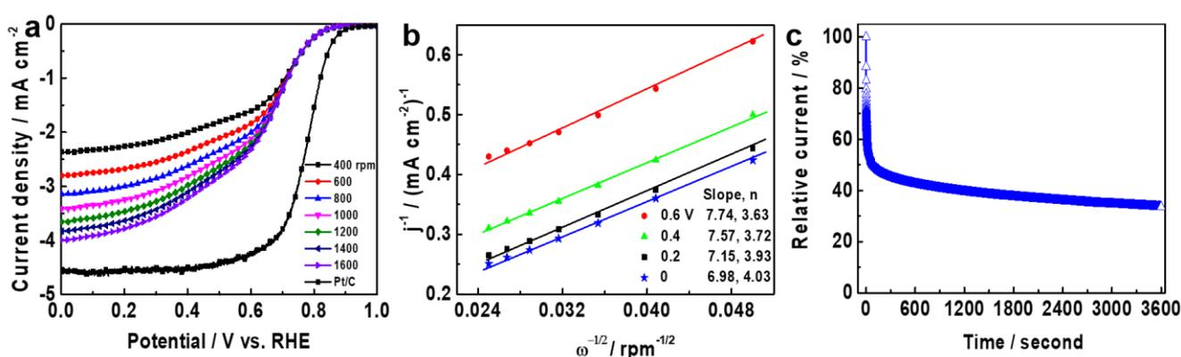
**Figure 4.** (a) LSV curves for ORR of Fe<sub>3</sub>-600 at various rotational rates and the LSV of commercial Pt/C (20% wt) at 1600 rpm, (b) K-L plots of Fe<sub>3</sub>-600, (c) stability for ORR of Fe<sub>3</sub>-600.
