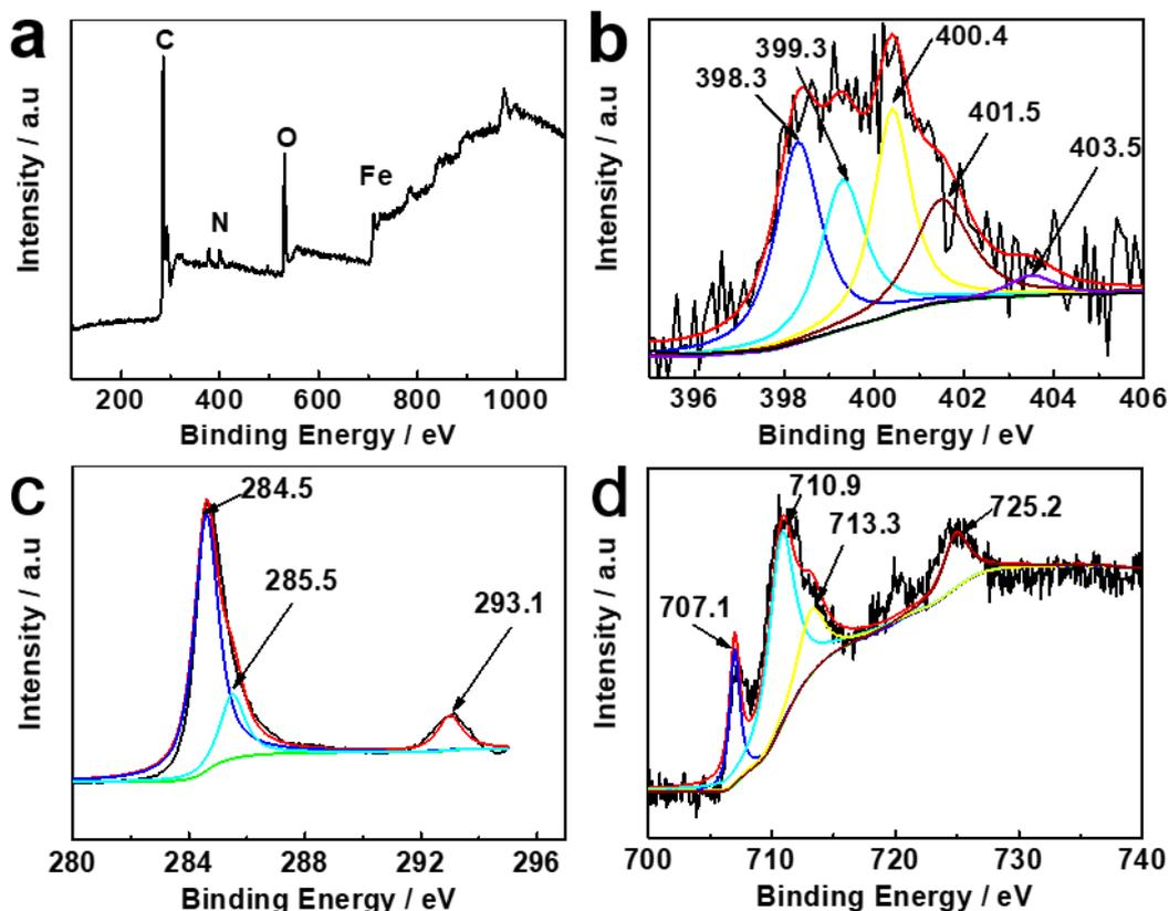
**Figure 8.** XPS survey spectra of Fe<sub>3</sub>-600, (a) survey, (b) N 1s, (c) C 1s, (d) Fe 2p.
