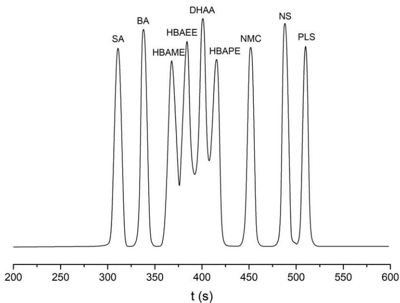
**Figure 5.** Electrophoretogram of nine preservatives in separation PBS (pH=6.0) at separation voltage 18 kV.
