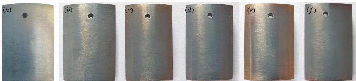
**Figure 7.** Macroscopic corrosion morphology of C71500 alloy after immersion in 3.5 wt.% NaCl + 0.5 wt.% Na<sub>2</sub>S solution at different temperatures (20, 25, 30, 35, 40 and 45°C) for 24 h: (a) 20°C; (b) 25°C; (c) 30°C; (d) 35°C; (e) 40°C; (f) 45°C.
